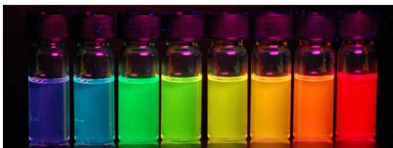
(left) Microdisk laser with colloidal quantum dots embedded, coupled to a single mode waveguide (middle,b) Microscopy images of the microdisk with the embedded quantum dots. (right) CdSe quantum dots in solution. The size increases from left (blue) to right (red) due to quantum confinement of the electron-hole pairs that emit light.
