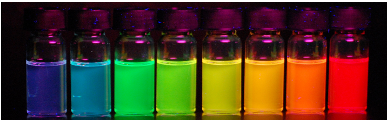
Figure (left) Two dimensional CdSe quantum wells obtained via wet chemical synthesis. The "plates" are 1.3 nm thick, with a lateral area of 34 x 15 square nanometers. (right) Luminescence of CdSe QDots under UV light, going from small (left, blue) to large (right, red) particles.
