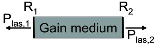
**Figure 3.1:** Schematic view of a semiconductor laser diode.
