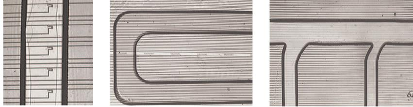
**Figure 5.11:** Pictures of PDMS microfluidics bonded to SOI chips with the stamp-and-stick procedure using an adhesive layer. Channel dimensions range from  $50 \times 50 \mu\text{m}$  to  $200 \times 50 \mu\text{m}$ .
