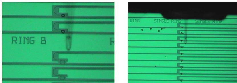
*Figure 1.4: SOI microring resonators of  $10 \times 14 \mu\text{m}$  area addressed separately with liquid drops of compatible dimensions produced with a Bioforce ‘Nanospotter’.*
