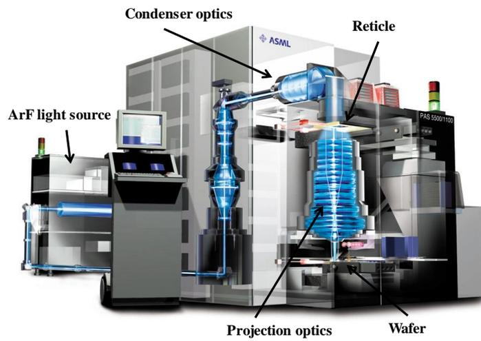
Figure 2.4: ASML PAS5500/1100.
