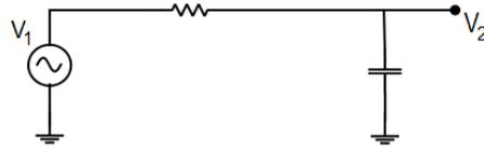
Figure 1.1: Lumped model of the interconnection between two transistors.
