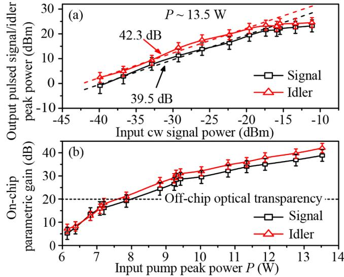
Figure 3.29: (a) Output pulsed signal/idler peak power v.s. input cw signal power at  $\lambda_s = 2356$  nm, with input pump peak power  $P \approx 13.5$  W. (b) On-chip parametric gain as a function of  $P$ . Off-chip optical transparency is achieved with a peak power of  $\approx 8$  W.
