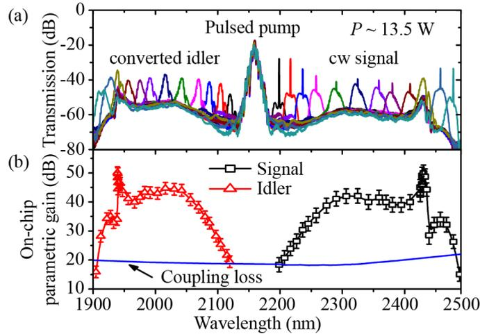
Figure 3.28: (a) Series of FWM spectra with the pulsed pump co-propagating with a cw mid-IR signal at various wavelengths. The pulsed pump is centered at  $\lambda = 2173$  nm, and has  $P \approx 13.5$  W. (b) Spectrum of on-chip parametric signal gain (black squares) and idler conversion gain (red triangles). Fiber-waveguide coupling loss measured with cut-back method is shown by the blue trace.
