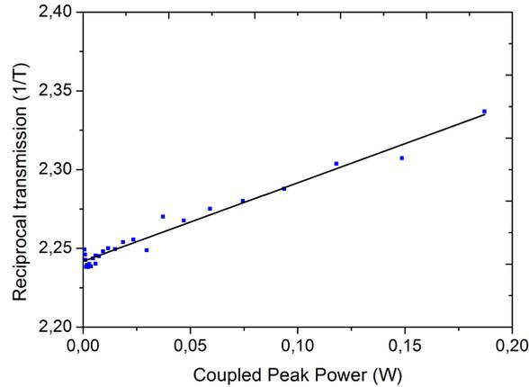
Figure 6.18: The reciprocal transmission as a function of the input peak power of the 4 ps pulse train. The linear fit corresponds to a nonlinear absorption coefficient of  $-28 \pm 3 \text{ W}^{-1}\text{m}^{-1}$ .
