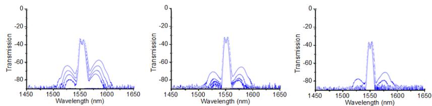
Figure 6.10: Modulation instability as a function of time for different temperatures. The three panels show the output spectrum of 4W peak pulses when the chip is held at room temperature (left), 80 °C (middle) and 120 °C (right). The spectrum is recorded after 1 min, 5 min, 20 min and 60 min for these three temperatures.
