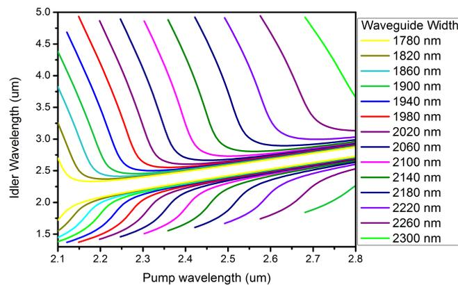
Figure 3.22: The phase matched idler and signal wavelength as a function of the pump wavelength for a set of silicon waveguides with a varying width and a height of  $400 \text{ nm}$  resting on a sapphire substrate.
