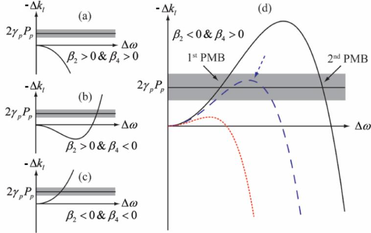
Figure 3.1: The phase mismatch as a function of detuning frequency. Depending on the sign of  $\beta_2$  and  $\beta_4$  the phase matching equations has several solutions. a)  $\beta_2 > 0$  and  $\beta_4 > 0$ , b)  $\beta_2 > 0$  and  $\beta_4 < 0$ , c)  $\beta_2 < 0$  and  $\beta_4 < 0$ , d)  $\beta_2 < 0$  and  $\beta_4 > 0$
