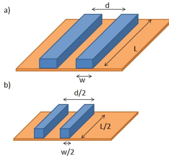
Figure 1.3: Easy model illustrating the effects on electric connections after scaling these down.
