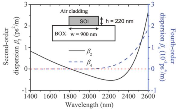
Figure 3.4: The group velocity dispersion and the fourth order dispersion as a function of wavelength.
