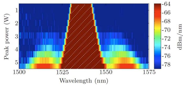
Figure 6.26: (Color online) MI spectra as a function of the input power, which is outside the range of the color coding at approximately  $-30\text{dBm/nm}$ .
