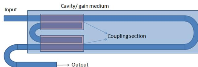
Figure 5.4: A schematic of a singly resonant monolithically integrated optical parametric oscillator.
