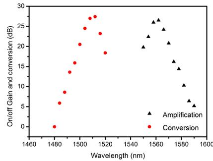
Figure 7: The amplification of the all-optical amplifier implemented in amorphous silicon. The amplification of the amplifier as a function of signal wavelength is shown.
