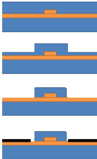
*Figure 7.8: The process flow to deposit metal contacts next to a rib waveguide. First the oxide is partially opened with a dry etch to remove most of the oxide, after which the remaining oxide is removed with a HF wet etch. Finally the metal is deposited.*
