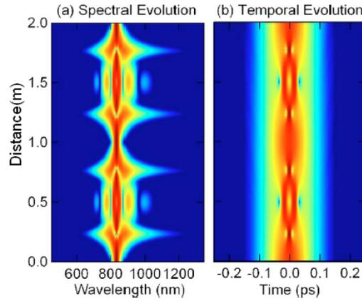
Figure 4.2: Periodic evolution of the spectral and temporal characteristics of the higher-order ( $N=3$ ) soliton in a nonlinear material pumped in the anomalous regime. The peak power of the pulse is 1250 W, its duration is 200 fs, while the nonlinearity of the photonic crystal fiber is assumed to be  $0.11 \text{ W}^{-1} \text{ m}^{-1}$ . The length unit has been normalized to the period of the higher order soliton. Figure from [7]
