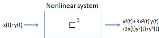
Figure 1.10: A nonlinear system. In a nonlinear system, the output is not a linear superposition of the outputs of signals presented to the system, some cross terms appear at the output as well.
