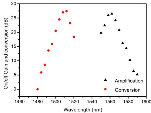
Figure 6.6: The conversion efficiency and amplification in a-Si:H waveguides. The figure shows the conversion efficiency and amplification as a function of the signal pulse wavelength when the coupled peak power of the pump pulses was 5.3 W in a 1 cm long waveguide.
