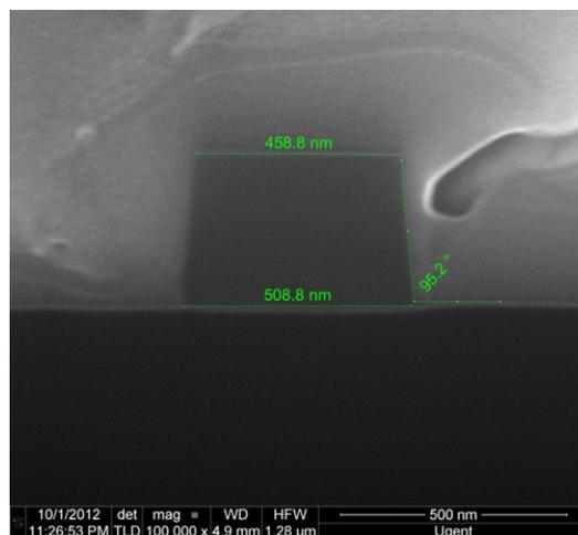
Figure 4.12: A cross section of a 400 nm high, 500 nm wide waveguide resting on a silicon oxide substrate. The side wall angle is almost 90 degrees. The clouds surrounding the waveguide are parts of the platina used while making the cross section
