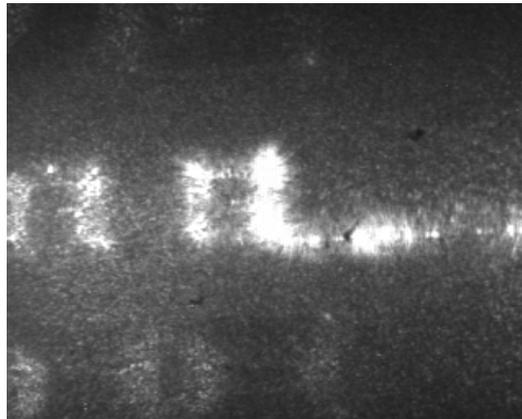
*Figure 6.15: telecommunication wavelength light is traveling through the fabricated spiral waveguides.*
