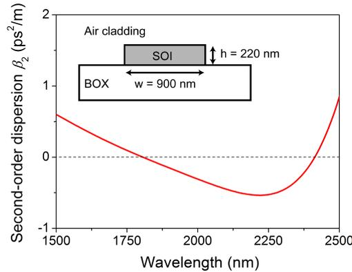
Figure 4.18: Group velocity dispersion of the silicon wire waveguide as a function of the wavelength, exhibiting anomalous dispersion ( $\beta_2 < 0$ ) between 1810 nm and 2410 nm. The inset shows the fabricated wire waveguide dimensions.
