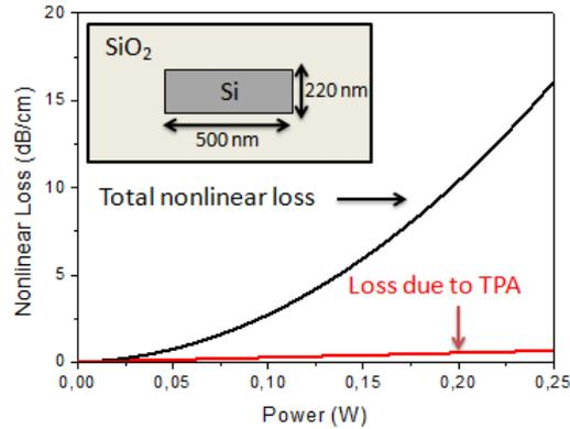
Figure 7.1: The nonlinear absorption of a silicon waveguide. The inset shows the dimensions of the waveguide used in the simulation. The graph shows the absorption in dB/cm as a function of the input power.
