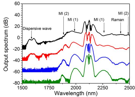
Figure 4.8: Measured output spectrum for increasing values of coupled input peak power: 3.1 W (green), 4.3 W (blue), 7.9 W (red) and 12.7 W (black). The spectra are vertically offset by multiples of 20 dB for clarity.
