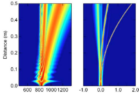
Figure 4.3: Results from numerical simulations showing spectral and temporal evolution for Raman induced fission of an incident  $N=3$  soliton. The pulse properties are similar as in the previous figure. Figure from [7]
