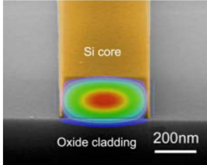
Figure 1.11: The mode profile in a silicon waveguide. The light is confined to a very small modal area. Courtesy of Dr. William Green from IBM T.J. Watson Research Center.
