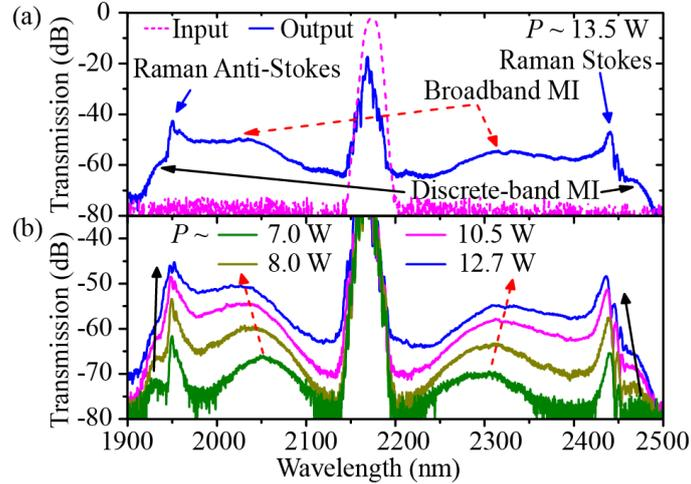
Figure 3.27: (a) Input (dashed magenta) and output (solid blue) pump spectrum, taken with an input peak power  $P \approx 13.5$  W and  $\lambda = 2173$  nm, illustrating ultra-broadband MI, and Raman Stokes/anti-Stokes peaks. (b) MI spectra with four different pump peak power levels at pump wavelength  $\lambda = 2173$  nm.
