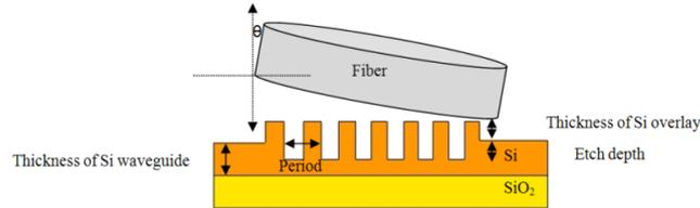
Figure 2.6: A schematic the designed grating coupler.
