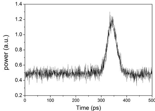
Figure 3.17: A trace showing the temporal evolution of the cw laser at 1565 nm. When the laser overlaps temporarily with the 19 W peak power pulses at 2190 nm, the cw signal gets amplified.
