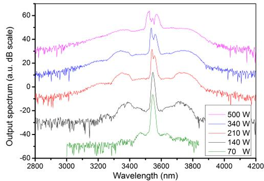
Figure 4.16: The output spectra of the 1 cm long, 1850 nm wide waveguide as a function of peak power when pumped at 3550 nm. At higher peak powers the facets of the waveguides got damaged.
