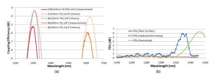
Fig. 6: Theoretically and experimentally obtained fiber-to-waveguide coupling spectra (a) and PDL (b) for the F(1310 nm - TE) B(1310 nm - TM) grating coupler design in Table lb.
