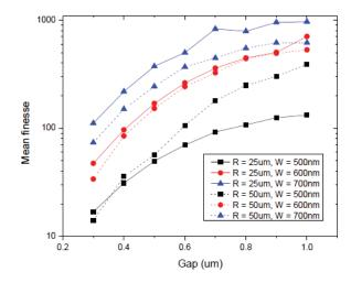
Figure 4.7: The mean finesse (1520nm-1560nm) over all resonances per ring as a function of gap for varying waveguide width (W) and radius (R). (Courtasy of Peter De Heyn [10])
