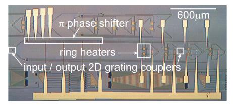
Figure 4.4: Microscope picture of a fabricated FlexPON WR SOI chip.
