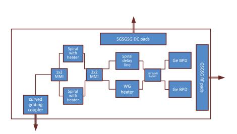
Figure 3.7: DQPSK receiver Silicon Photonics circuit layout. The arrows are the probing direction of a component.
