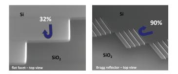
Figure 2.25: Planar concave grating reflectors with flat facet (left) and DBR facets (right). (Courtasy of Joost Brouckaert [33])
