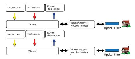
Figure 2.9: Optical equipment needed for two customers using discrete components and packaged in two separate SFP packages.
