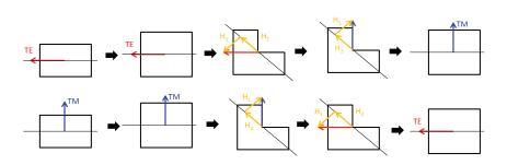
Figure 3.16: Polarization rotator principle explanation using the waveguide cross sections and electrical fields of the modes.
