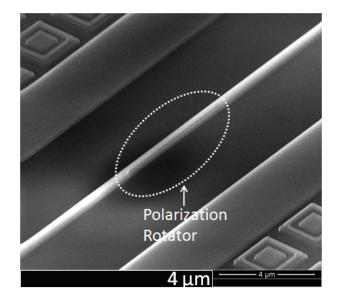
Figure 3.15: Bird's eye view SEM image of a fabricated polarization rotator.
