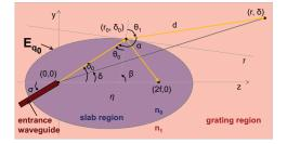
Fig. 1. Focusing grating coupler geometry parameters. The light (yellow arrows) is refracted and reflected at the first grating ellipse  $E_{q_0}$ .  $\tau$  and  $\eta$  are the tangent and normal line respectively of ellipse  $E_{q_0}$  at point  $(r_0, \delta_0)$ .
