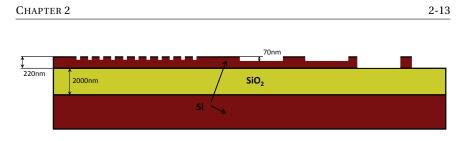
Figure 2.12: Imec<sup>1</sup> passive platform. A Silicon-on-Insulator (SOI) wafer with 2 µm Buried Oxide (BOX) layer and 220 nm silicon waveguide core with a 220 nm deep etch and 70 nm shallow etch.
