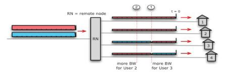
Figure 4.9: Downstream data following the FlexPON principle.
