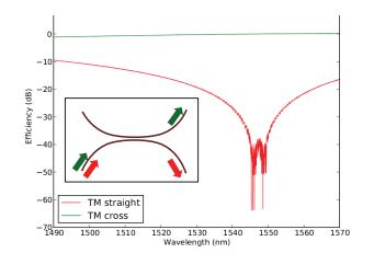
Figure 3.13: Measured efficiency for the polarization splitting directional coupler when the TM-polarized mode is launched.
