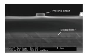
Figure 2.17: Cross-section SEM image of the fabricated grating coupler with DBR bottom mirror.
