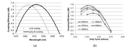
*Figure 2.14: The spectrum (a) of grating couplers using a Silicon overlay spectrum. The top efficiency as a function of the duty cycle for different grating periods (b).*
