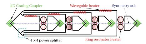
Figure 4.3: Polaization diversity implementation of a FlexPON WR. 2D grating couplers are used as in and out coupling elements. The upper circuit introduces a  $\pi$  phase shift using thermally tunable waveguide heaters for PDL minimization.
