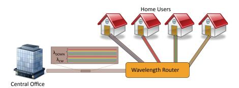
Figure 4.1: Schematic drawing of a FlexPON newtork. A reconfigurable wavelength router (part of the RN) drops wavelength pairs from the Central Office to the Home Users or ONU.
