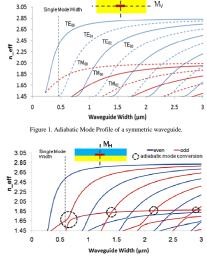
Figure 2. Adiabatic Mode Profile of an asymmetric waveguide.
