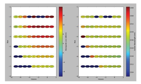
Figure 2.30: Wafer-scale automated testing of quarter wafer. The waveguide loss of a single-mode waveguide and central wavelength of standard test grating couplers are plotted as a function of the row and column number.
