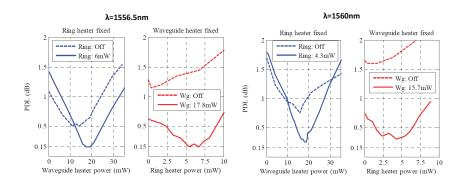
Figure 4.5: PDL measurements of the FlexPON WR chip as a function of the waveguide and ring heater power for two different wavelengths. (see [3] on page 4-15)
