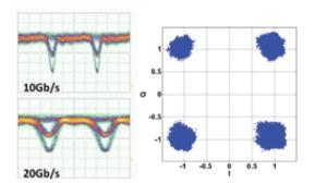
Figure 3.9: Eye diagrams and symbol diagram for the DQPSK transmitted signal.
