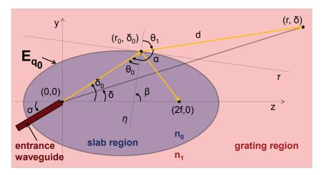
Figure 4.13: Focusing grating coupler geometry parameters. The light (yellow arrows) is refracted and reflected at the first grating ellipse  $E_{q_0}$ .  $\tau$  and  $\eta$  are the tangent and normal line respectively of ellipse  $E_{q_0}$  at point ( $r_0$ , $\delta_0$ ).
