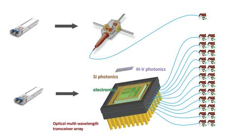
Figure 2.3: Optical integration enables multiple transceivers (12/24) in an SFP package.
