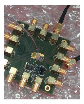
Figure 2.34: 8-channel fiber array attachement with UV-curable epoxy.
