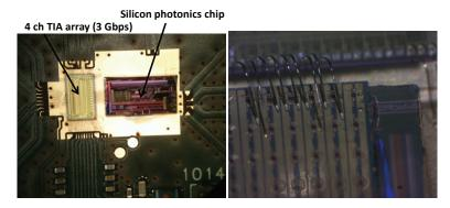
(a) SOI chip wirebonded to a PCB board and (b) Zoom-in picture of wirebonds from the a 4-channel 3Gb/s TIA array.
