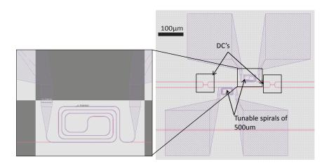
Figure 3.2: Mask design of a tunable MZI splitter optimized for e-beam lithography.
