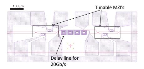
Figure 3.3: Mask design of a DPSK receiver with tunable MZI splitter and combiner for e-beam lithography. The delay line is sectionized such that the number of writing field intersections is minimized.
