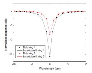
Figure 4.8: Illustration of two critically coupled microring resonators with a Lorentzian fit. Ring 1:  $R = 25 \mu m$ , gap = 0.7  $\mu m$ , width = 0.7  $\mu m$ , around 1550nm. Ring 2:  $R = 50 \mu m$ , gap = 0.7  $\mu m$ , width = 0.7  $\mu m$ , around 1530 nm. (Courtasy of Peter De Heyn [10])
