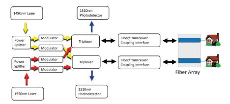
Figure 2.10: Integration scheme for 2-channel FTTH transceiver array using on-chip lasers, modulators and photodetectors.
