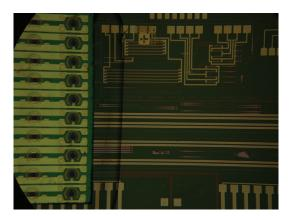
Figure 2.32: Picture of silicon chip demonstrator with SU8 epoxy attached III/V transparent photodetector array.
