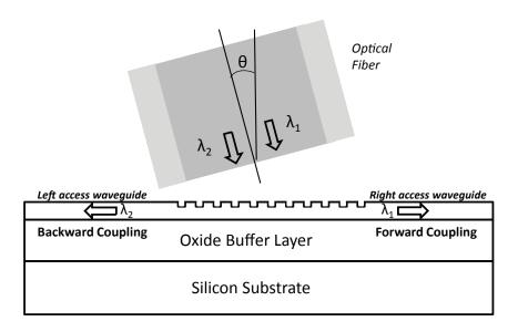
Figure 2.18: Working principle of grating duplexer.
