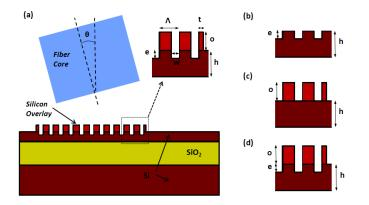
Fig. 2. Parameterized highly directional grating couplers: the general case (a), without silicon overlay (b), with silicon overlay but no waveguide etch (c) and both silicon overlay and waveguide etch (d).
