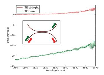
Figure 3.12: Measured efficiency for the polarization splitting directional coupler when the TE-polarized mode is launched.
