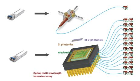
Figure 5: SFP package containing one FTTH transceiver using discrete optics (top) and 24 FTTH transceivers (bottom) using Silicon Photonics technology.
