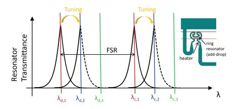
Figure 4.2: The spectrum before and after tuning of a microring resonator. The Free Spectral Range (FSR) coincides with the wavelength spacing between the Downstream (DS) and Continuous Wave (CW) wavelength pairs.
