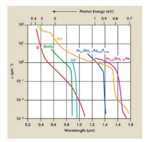
Figure 2.20: Absorption spectra of different materials.
