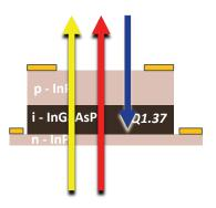
Figure 2.21: Cross section of the transparent photodetector. The InP layers and quaternary layer thicknesses are optimized for transparency of the upstream wavelengths 1490 nm and 1550 nm.
