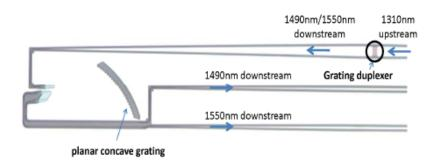
Figure 2.24: Microscope image of a grating duplexer in combination with a Planar Concave Grating (PCG) demultiplexer splitting 1490 nm and 1550 nm.
