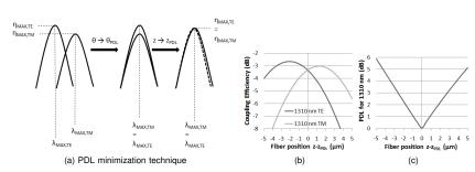
Fig. 5: PDL minimization technique and alignment sensitivity plots for the optimized  $F(1310 \text{ nm} - TE) B(1310 \text{ nm} - TM) - (9^{\circ})$  grating using a silicon overlay.
