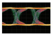
Figure 2.37: Channel 3 1310 nm transparent photodetector eye diagram at 1.25 Gb/s and PRBS of  $2^7 - 1$ .
