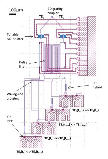
Figure 3.17: Mask design of a PM-DQPSK receiver using a polarization tracking architecture.
