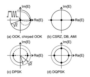
Figure 3.1: Modulation formats symbol diagrams: On-Off Keying (a), Duobinary (b), Differential Phase Shift Keying (C) and Differential Quadrature Phase Shift Keying (d). (Courtasy of Peter Winzer [1])
