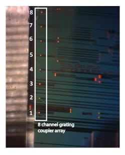
Figure 2.29: Picture of the Silicon Photonics chip for the 4-channel FTTH transceiver array demonstrator. The chip was illuminated under an angle.
