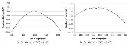
Fig. 3: Measured coupling efficiency of the  $F(1310\,{\rm nm}-TE)\,B(1520\,{\rm nm}-TE)-(10\,^{\circ})$  grating duplexer.
