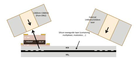
*Figure 2.22: Silicon photonics circuit with integrated transparent photodector on a grating coupler.*
