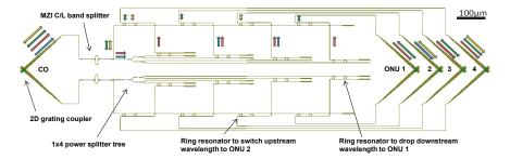
Figure 4.12: Mask design of a wavelength router enabling a XPON/FlexPON network architecture. The ring and waveguide heaters are not shown for clarity.
