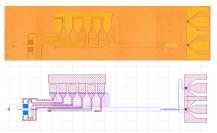
Fig. 1. Design of the differential receiver for DQPSK and 10G symbol rate (upper) optical photograph of fabricated device, (lower) gds design. The receiver is assembled using 5 componentes, from left to right in the figure Curved grating coupler, M2I tunable power splitter, delay-line interferometer, 90-degree hybrid and two balanced photo detectors.
