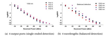
Figure 3.6: BER vs. received power measurements. (courtesy of Nikolaos Sotiropoulos)
