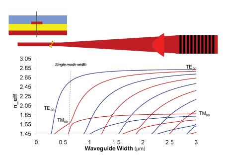
Figure 2.19: Effective refractive index of the waveguide modes as a function of the waveguide width. The fundamental TM mode couples to higher order TE modes when the waveguide width is decreased. (blue lines = even modes, red lines = odd modes)
