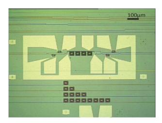
Figure 3.4: Microscope picture of a fabricated DPSK receiver with e-beam lithography.
