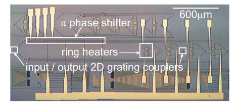
Figure 8: Microscope picture of a fabricated FlexPON wavelength router SOI chip.
