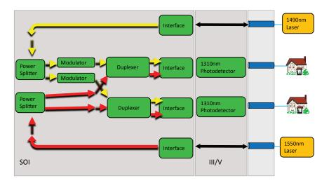
Figure 2.23: 2-channel FTTH transceiver layout using transparent photodetectors to detect the 1310 nm downstream band.
