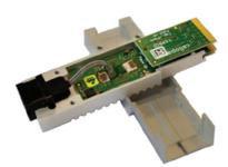
Figure 2.38: 12-channel commercial FTTH transceiver product from Caliopa (imec/UGent Silicon Photonics startup) using similar transparant photodetector technology pioneered in this work.
