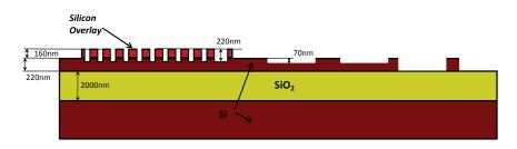
Figure 2.13: Imec<sup>1</sup>'s advanced passive platform. A Silicon-on-Insulator (SOI) wafer with 2 µm BOX layer and 220 nm silicon waveguide core and 160 nm amorphous/poly-Si overlay layer. Different etch depths of 230 nm, 70 nm and 220 nm can be used.
