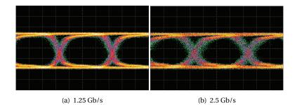
Figure 2.36: Measured modulator eye diagrams at 1510 nm and for a PRBS of  $2^{31} - 1$ achieving an ER of 17 dB.
