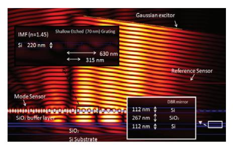
Figure 2.16: Simulated field profile of grating coupler with Bragg bottom mirror.
