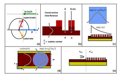
Fig. 1. Schematic illustrations of fiber-to-chip high index contrast grating coupler optimization factors: the Bragg condition (a), upwards directionality (b), 2D fiber mode-matching in z- and x-direction (c,d) and mode-matching between the waveguide and Bloch mode of the grating (e).
