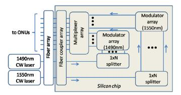
Figure 2.27: Silicon chip configuration for the integrated transceiver arrays for FTTH CO equipment.
