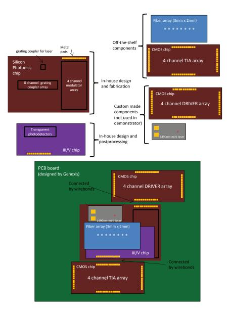
Figure 2.28: General layout of the 4-channel FTTH transceiver array demonstrator. A III/V chip and mini laser are attached to the Silicon Photonics chip using an epoxy. This chip is mounted on a pcb board wirebonded to a driver and TIA chip. An 8-channel fiber array is actively aligned and attached to the chip.
