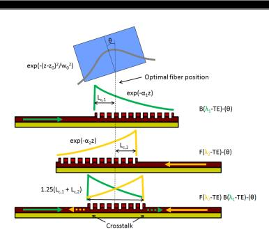
Fig. 2: Mode-matching for uni-directional and bi-directional grating couplers.
