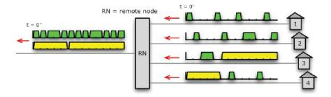
Figure 4.11: Modulated upstream signals combined at remote note.
