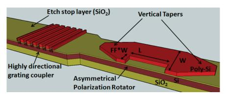
*Figure 3.14: Artist's impression of a highly directional fiber coupler and asymmetrical polarization rotator fabricated within the same process flow. (Dimensions are not to scale)*
