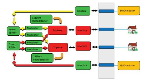
Figure 2.11: Integration scheme for 2-channel FTTH transceiver array using on-chip modulators and photodetectors. The lasers are external pigtailed lasers.
