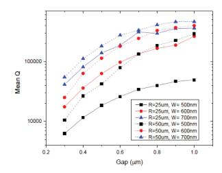
Figure 4.6: The mean Q<sub>i</sub> (1520 nm – 1560 nm) of shallow rib waveguide based ring resonators as a function of gap for varying waveguide width (W) and ring radius (R). (Courtasy of Peter De Heyn [10])
