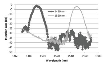
Figure 2.26: 2-channel PCG demultiplexer insertion loss spectra.
