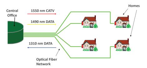
Figure 2.1: Optical wavelengths used in a Fiber-To-The-Home PTP triple-play network.
