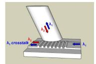
Figure 2: Operation principle of a grating duplexer.  $\lambda_1$ represents the upstream wavelength band,  $\lambda_2$ represents the downstream wavelength band.
