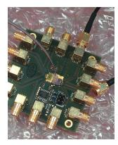
Figure 6: 4-channel FTTH transceiver demonstrator, developed in cooperation with Genexis, Caliopa and the Technical university of Eindhoven in the framework of the Dutch Smartmix-Memphis project.
