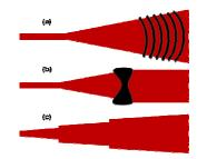
Figure 3. Non-Adiabatic tapers: (a) Focusing Grating Coupler (b) Lensed Focusing Taper (c) Discontinuous Taper
