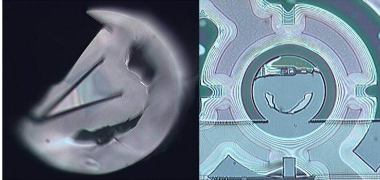
**Figure 3.12:** Bad detachment of the photonic circuit membrane after collapse. Part of the photonic circuit is stuck to the fiber facet (left) while other part remains on the SOI chip (right).
