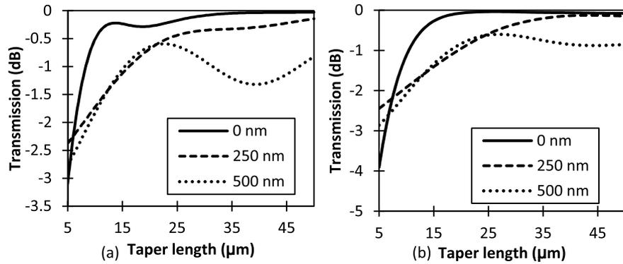
**Figure 2.19:** Transmission for the fundamental TE-mode through respectively (a) a linear taper design and (b) a piecewise linear taper design, for an alignment error of 0 nm, 250 nm and 500 nm, as a function of taper length.
