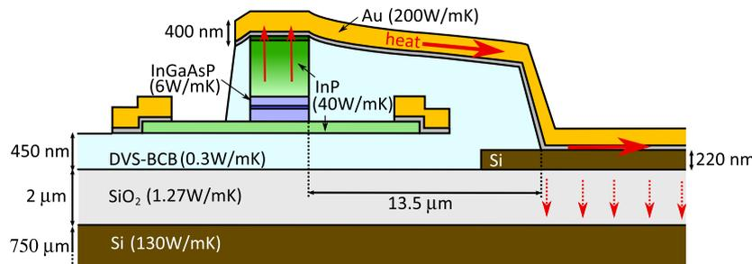
**Figure 2.7:** Thermal design used in the simulation.
