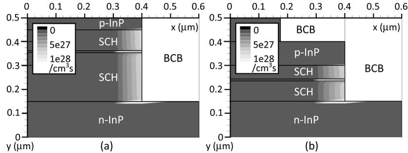
**Figure 2.9:** SRH and surface recombination rate ( $\text{cm}^{-3}\text{s}^{-1}$ ) in the (a) classical design and (b) the gallery design.
