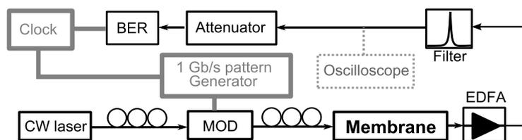
Figure 4.9: Experimental setup of BER measurement for the first generation devices.
