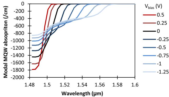
**Figure 2.21:** Modal absorption spectrum of the MQW structure with n-doped SCH layer as a function of wavelength, for different applied bias voltages across the device.
