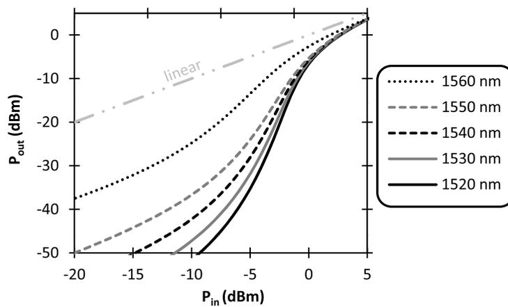
Figure 4.8: Simulation of static transmission through a 150  $\mu\text{m}$  long membrane.
