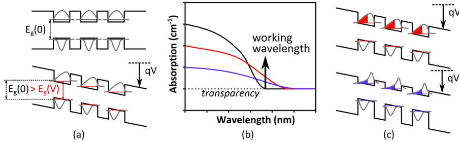
**Figure 2.11:** Principle of QCSE. (a) The reduction of the band gap and the shifting of the wave functions (grey) when applying a high electric field. (b) The absorption profile for the original case (black), and for an applied electric field for a large (red) and small (blue) conduction band discontinuity. (c) The band diagram under electric field for large and small conduction band discontinuity. The shaded area suggests the amount of overlap between the hole and electron wave functions.
