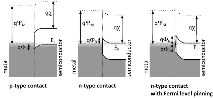
**Figure A.3:** Band diagram for metal-semiconductor contacts: p-type contact, n-type contact and n-type contact with Fermi level pinning.
