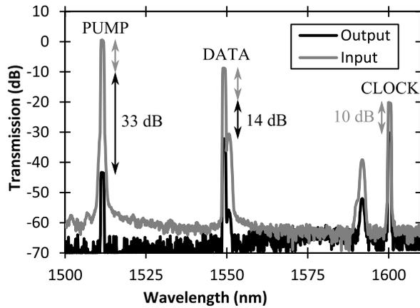
**Figure 5.18:** Input and output spectrum of pump, data and clock signal through single gate. The grey arrow marks the insertion loss, the black arrows mark the absorption loss in the gate.
