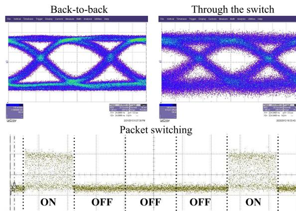
**Figure 5.26:** Top: eye diagram before and after switching. Bottom: trace of data where only one out of four packets is sent to the output port.
