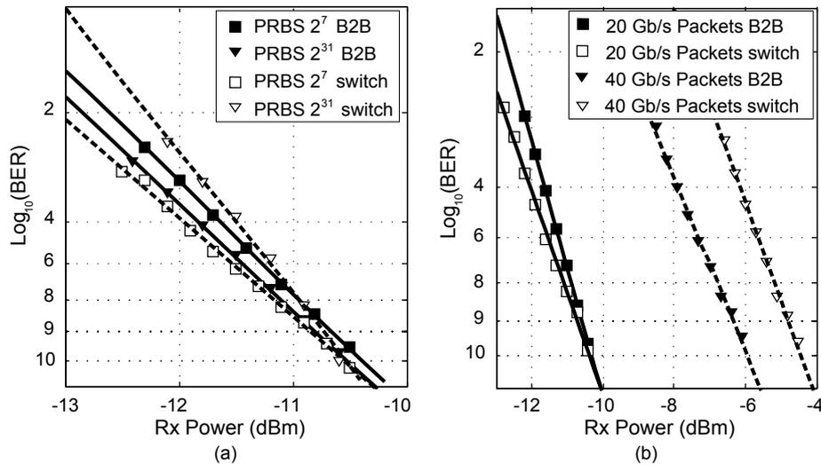
**Figure 5.13:** BER measurements through a single gate. (a) BER curves for a back-to-back and through the gate measurement for different pattern lengths. (b) BER curves for back-to-back and through the gate measurement at both 20 Gbit/s and 40 Gbit/s.
