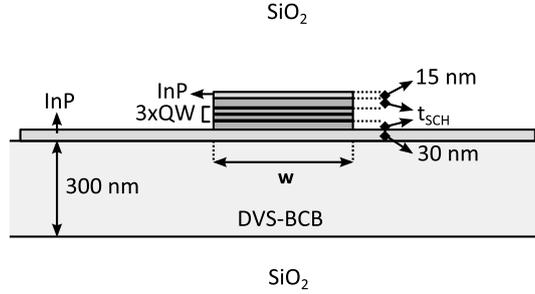
**Figure 3.14:** Schematic of waveguide that will be simulated.
