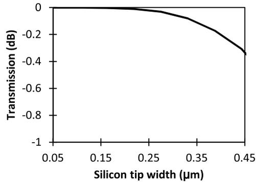
**Figure 2.18:** Effect of the silicon tip width on the device transmission of the fundamental TE-mode.
