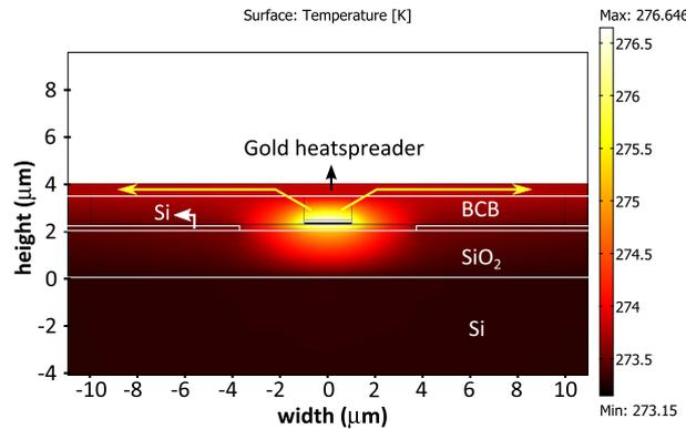
**Figure 3.6:** Thermal profile for the ridge waveguide with top gold heat spreader. The yellow arrows show the additional pathway along which generated heat can escape.
