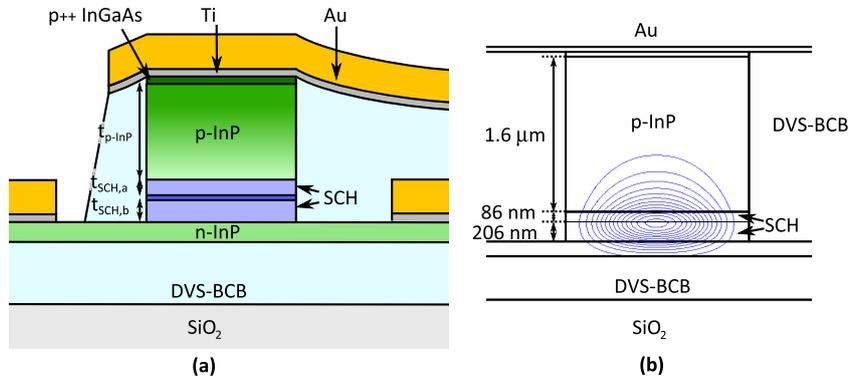
**Figure 2.1:** (a) Basic layout of the classical waveguide structure used on the heterogeneously integrated III-V/SOI platform. (b) Mode profile in the optimized waveguide.
