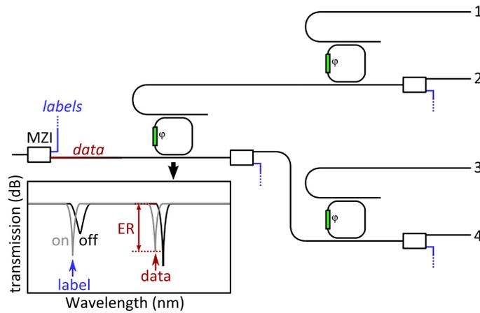
**Figure 5.6:** Schematic of implementation of resonator architecture using III-V membrane as phase section. The MZIs are used to (de)multiplex the label and data wavelength bands.
