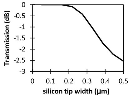
**Figure 3.9:** Transmission as a function of silicon tip width for a III-V width of 1  $\mu\text{m}$ .
