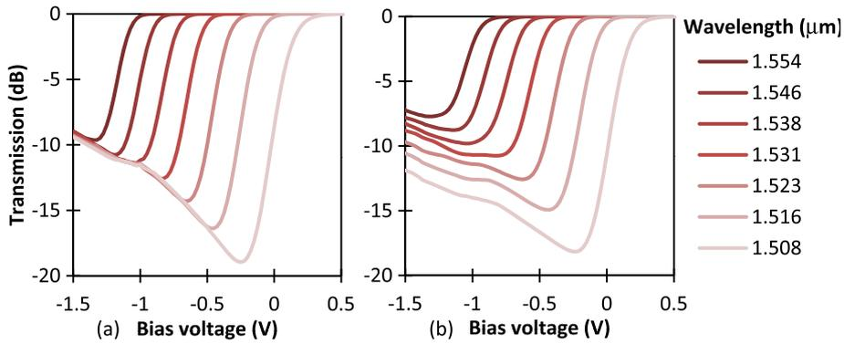
**Figure 2.23:** Simulated transmission through a modulator of respectively (a) 40  $\mu\text{m}$  long using the p-waveguide, and (b) 55  $\mu\text{m}$  long using the n-waveguide.
