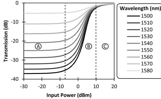
**Figure 4.2:** Transmission as a function of signal input power and signal wavelength.
