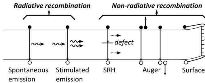
**Figure A.2:** Schematic overview of the different carrier generation and recombination processes.
