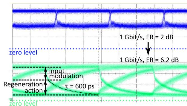
**Figure 4.12:** Measured eye diagram at 1 Gbit/s before and after regeneration at optimum regeneration conditions at a wavelength of 1530 nm.
