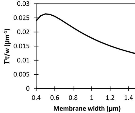
**Figure 4.3:** Efficiency of the regenerator as a function of the membrane width.
