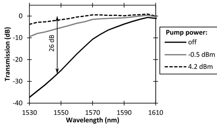
**Figure 5.17:** CW transmission through the gate used for the clock distribution experiment.
