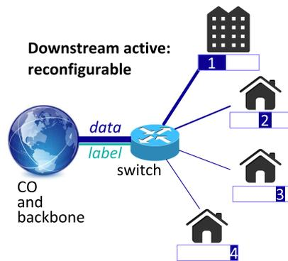
**Figure 5.3:** Schematic of typical active solution. Each connected ONU only receives the data meant for that ONU.
