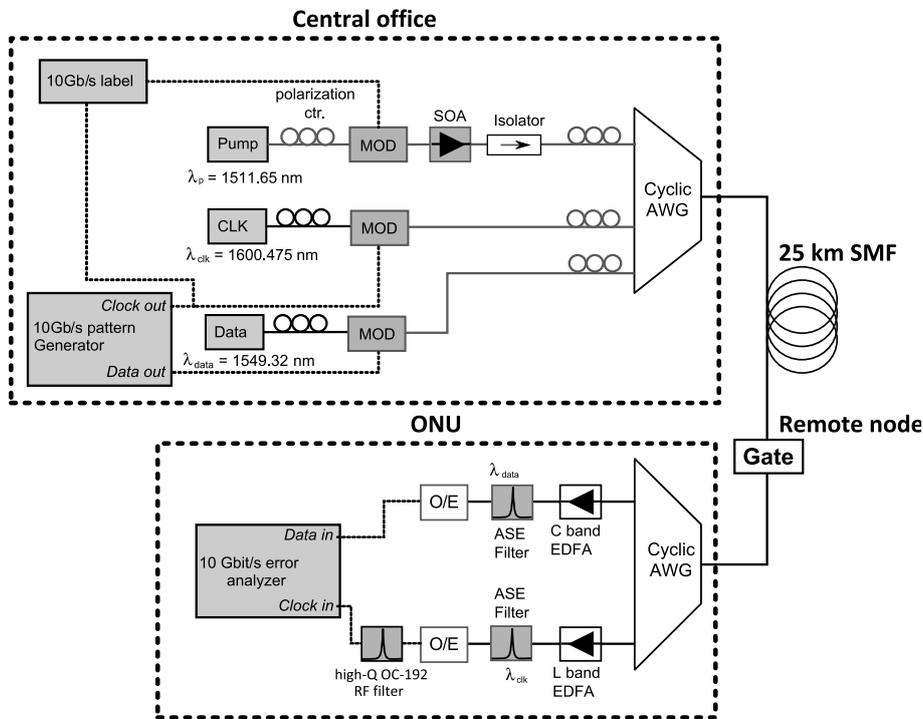
Figure 5.16: Setup for single gating experiment with clock distribution.
