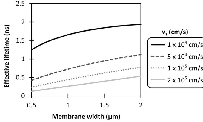
**Figure 3.13:** Influence of the surface recombination velocity  $v_s$  and the device width  $w$  on the effective carrier lifetime.
