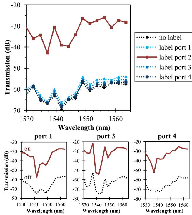
**Figure 5.23:** Static transmission through 1x4 switch. A high port isolation is demonstrated for all ports.
