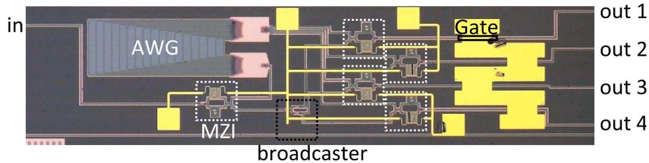
**Figure 5.21:** Optical microscopy image of fabricated 1x4 switch.
