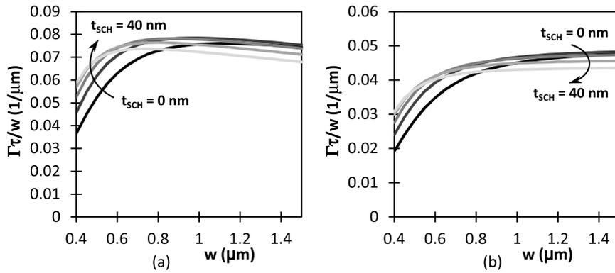
**Figure 3.16:** Simulated efficiency  $\Gamma\tau/w$  as a function of the membrane width  $w$  and SCH layer thickness  $t_{SCH}$  around the triple QW structure (a) for  $v_s = 1 \times 10^5$  cm/s, and (b) for  $v_s = 2 \times 10^5$  cm/s.
