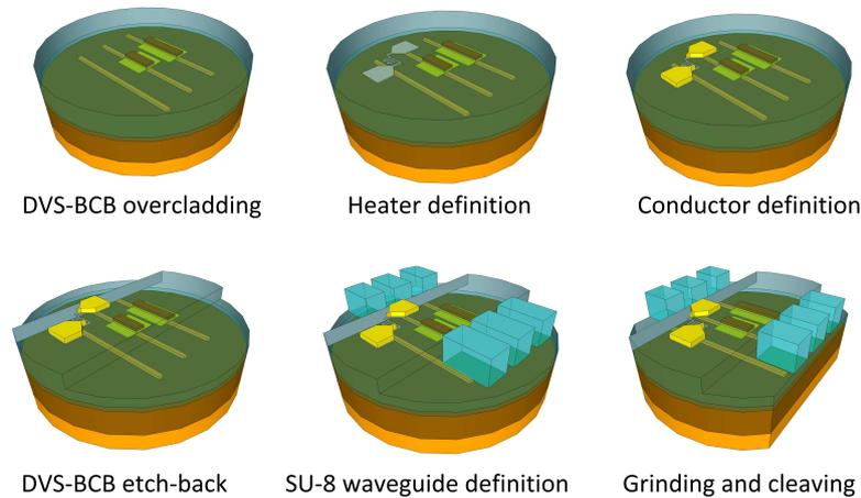
**Figure 3.19:** Fabrication recipe: heaters and couplers.
