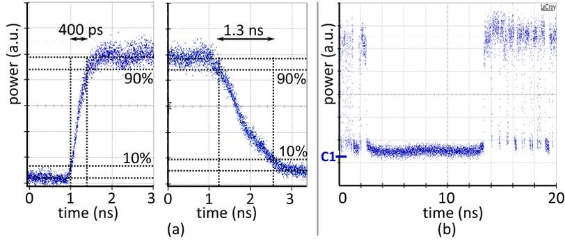
**Figure 5.14:** (a) Trace of gate switching on and off. (b) Trace of two packets with a switching window in between.
