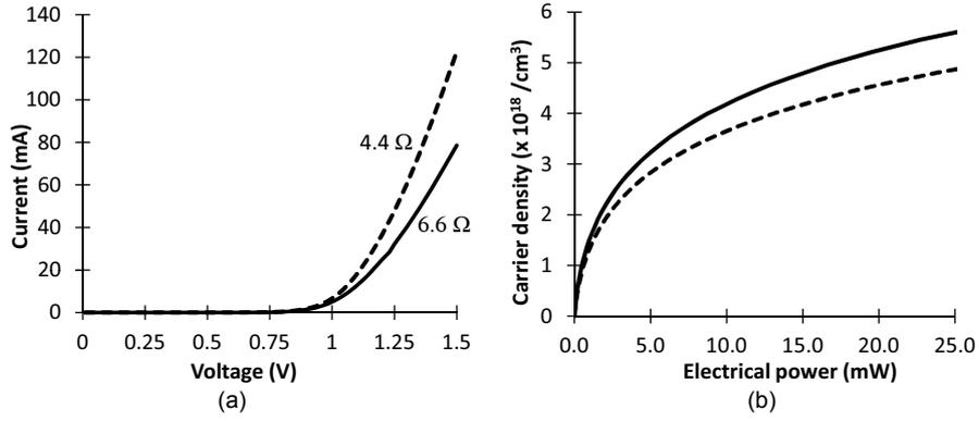
**Figure 2.8:** I(V) curve for the classical (dashed line) and gallery (solid line) design. The gallery has a higher series resistance, because of the reduced top contact area. (b) Achieved carrier concentration in the QW as a function of electrical power for the classical (dashed line) and gallery (solid line) design.
