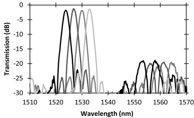
**Figure 5.11:** Transmission of the improved AWG design.
