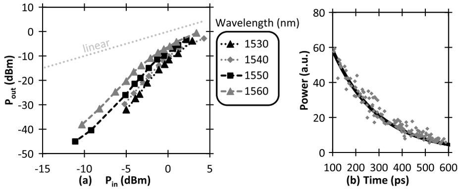
**Figure 4.13:** (a) Static transmission through the 2nd generation device. (b) Measurement of the roll-off of the probe transmission (grey), and fitted exponential (black) with  $\tau_{eff} = 200$  ps.
