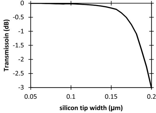
**Figure 3.11:** Influence of the silicon tip width on the SU-8 taper performance.
