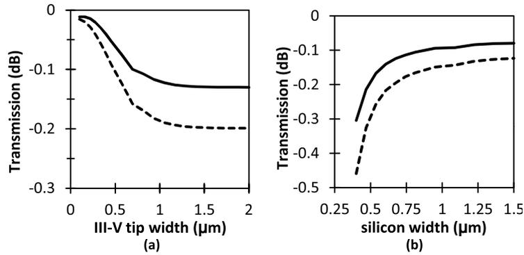
**Figure 3.8:** (a) Transmission as a function of III-V tip width for a silicon wire width of 700 nm. (b) Transmission as a function of silicon wire width for a III-V tip width of 1  $\mu\text{m}$ . The dashed curve corresponds to the situation with a strip waveguide, while the solid curve corresponds to the situation with a ridge waveguide.
