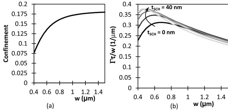
**Figure 3.15:** (a) Confinement as a function of membrane width  $w$ . (b) Simulated efficiency  $\Gamma\tau/w$  as a function of the membrane width  $w$  and SCH layer thickness  $t_{SCH}$  around the triple QW structure for  $v_s = 1 \times 10^4$  cm/s.
