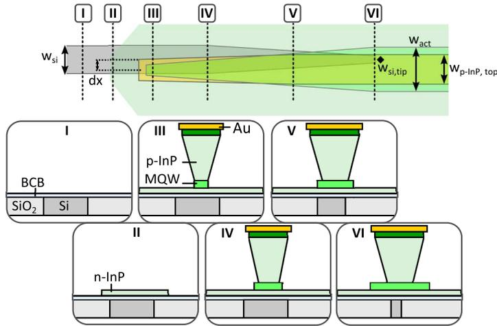
**Figure 2.16:** Basic layout of the inverted taper structure used to couple between the V-waveguide and the silicon wire. The parameter  $dx$  is the misalignment in the taper, which can occur during processing. In the ideal case, this should be 0 nm.
