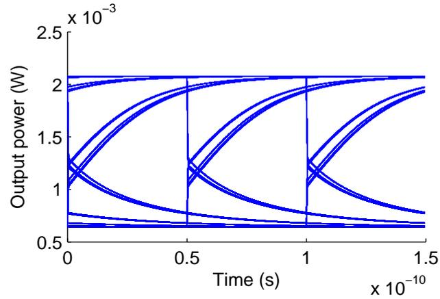
Figure 4.6: Simulated eye diagram at a bit rate of 20 Gbit/s.
