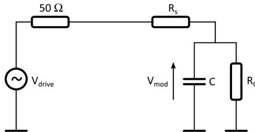
**Figure 2.24:** Small signal schematic of modulator driven by lumped electrodes.
