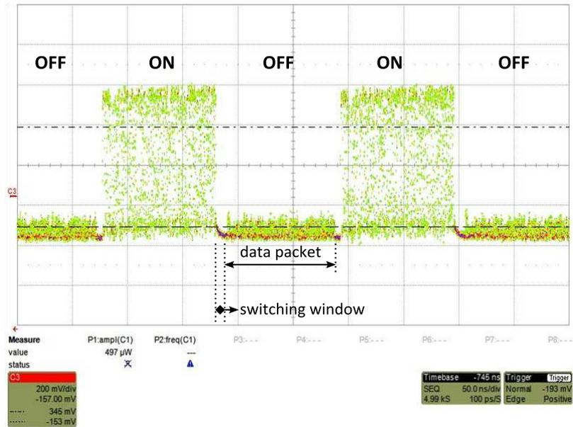
Figure 5.19: Trace of data packets after transmission through a switched on and switched off gate.
