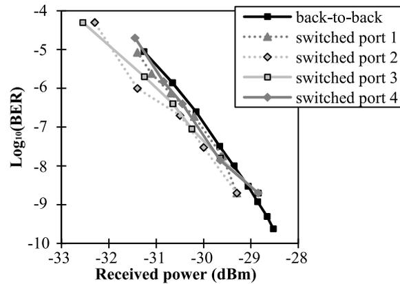
Figure 5.25: BER measurement for the 1x4 switch.
