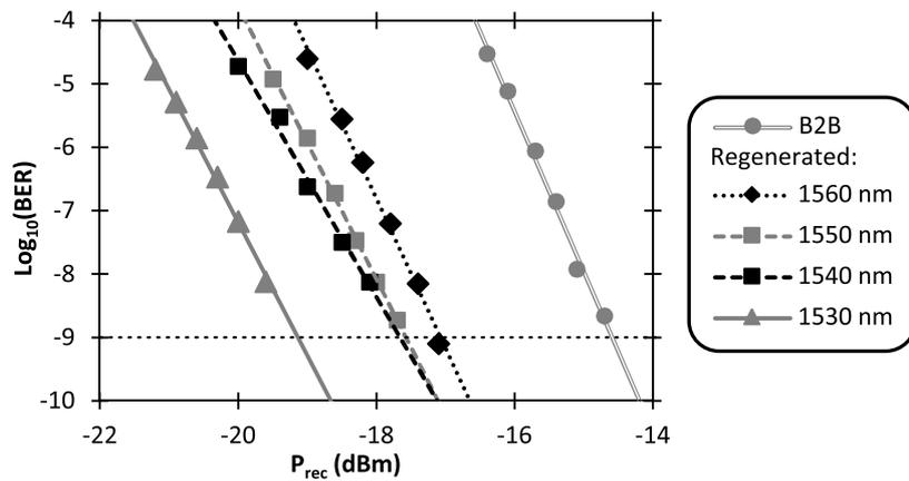
**Figure 4.11:** Comparison of the B2B BER measurement and the regenerated BER measurement in the 1530-1560 nm wavelength range.
