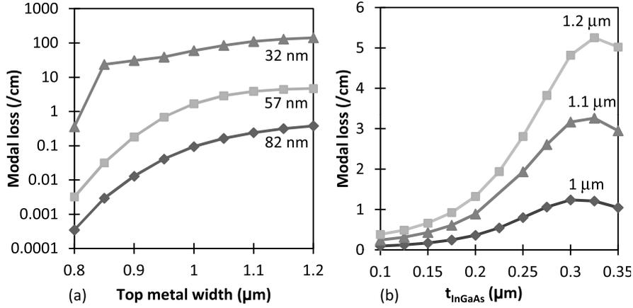
**Figure 2.15:** (a) Modal loss due to the contacting layers of the fundamental TE-mode as function of top metal width, for different values of the bottom SCH layer thickness. (b) Modal loss due to the contacting layers of the fundamental TE-mode as function of  $t_{\text{InGaAs}}$ , for different values of the top metal width. The loss has a peak for a InGaAs thickness of 300 nm, due to the effective index matching between the lossy mode near the metalization layers and the fundamental TE-mode.
