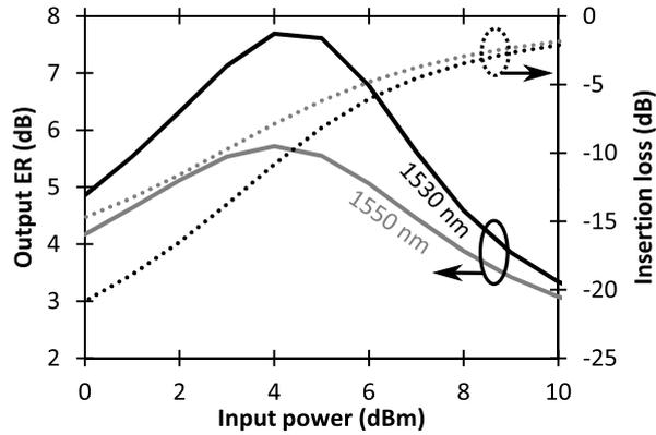
**Figure 4.4:** Output ER (solid line) and insertion loss (dotted line) of a 1530 nm (black) and 1550 nm (grey) signal with an input ER of 2 dB.
