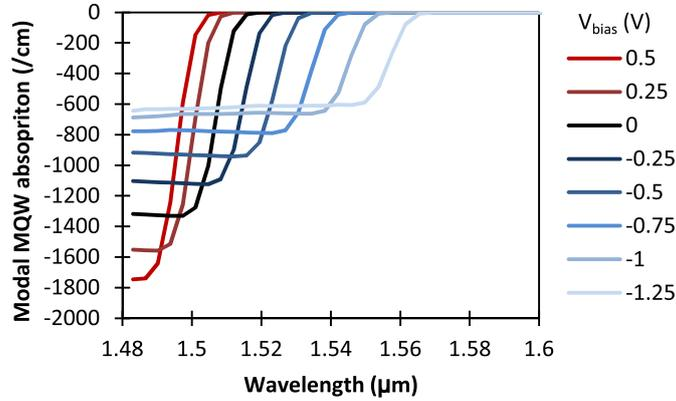
**Figure 2.22:** Modal absorption spectrum of the MQW structure with p-doped SCH layer as a function of wavelength, for different applied bias voltages across the device.
