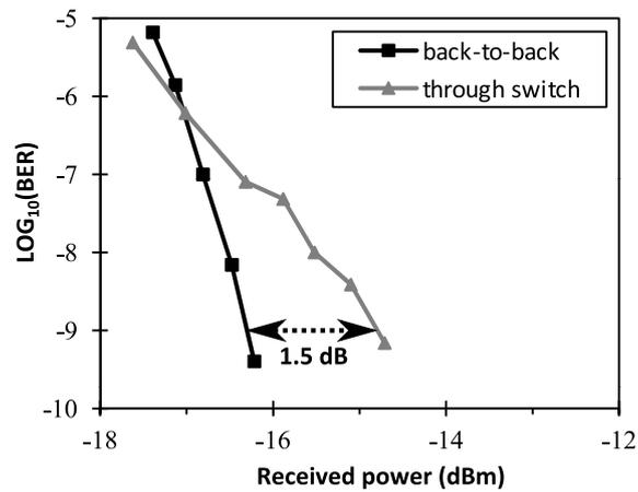
Figure 5.20: BER measurement results using the optical clock distribution.
