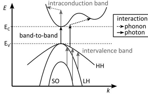
**Figure A.4:** Simplified band diagram of a direct semiconductor, showing the different absorption mechanisms.
