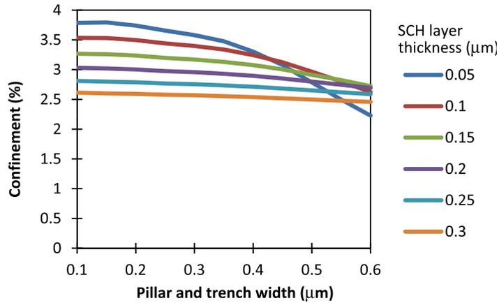
**Figure 2.5:** Confinement in the QW as a function of pillar and trench width, and SCH layer thickness.
