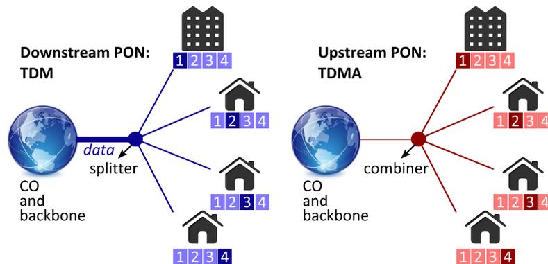
**Figure 5.1:** schematic of PON solution. A different wavelength is used for downstream and upstream data.
