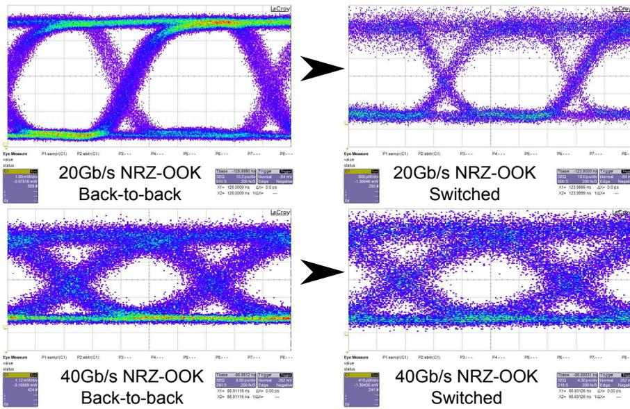
**Figure 5.15:** Eye diagrams for both the back-to-back and through the switch case at both 20 Gbit/s and 40 Gbit/s.
