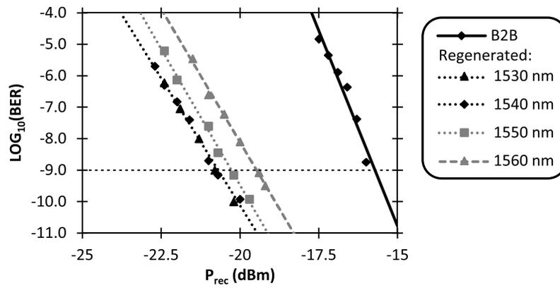
**Figure 4.15:** Comparison of the B2B BER measurement and the regenerated BER measurement in the 1530-1560 nm wavelength range.
