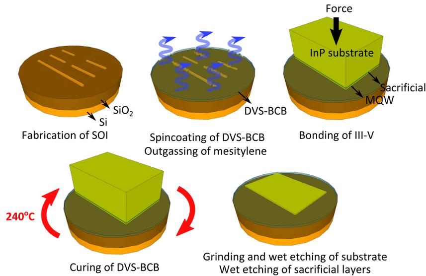
**Figure 3.17:** Fabrication recipe: preparation and bonding.
