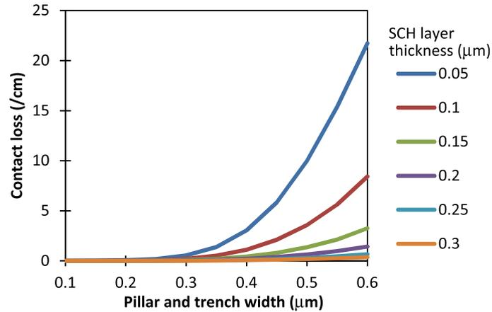
**Figure 2.4:** Losses due to absorption in the p-contact as a function of pillar and trench width, and SCH layer thickness.
