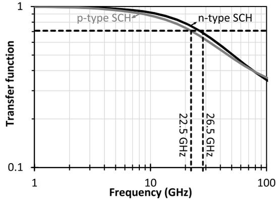
**Figure 2.25:** Device transfer function for a device length of 110  $\mu\text{m}$  and 125  $\mu\text{m}$ , for p-waveguide (grey) and n-waveguide (black) respectively.
