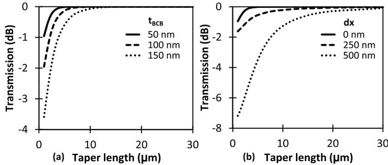
**Figure 3.10:** (a) Influence of the DVS-BCB thickness on the required taper length for adiabatic mode conversion ( $dx = 0$ ). (b) Influence of the alignment accuracy on the taper length for adiabatic mode conversion ( $t_{BCB} = 50$  nm).
