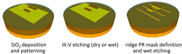
**Figure 3.18:** Fabrication recipe: patterning and etching of the membrane.
