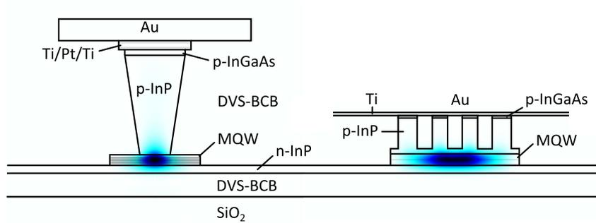
**Figure 4:** Proposed electrically injected waveguides: the V-waveguide (left) and the gallery waveguide (right).
