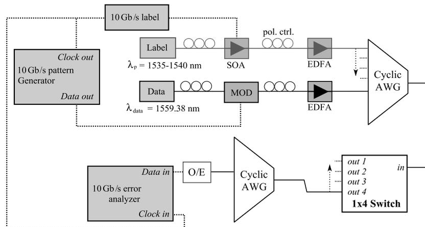
**Figure 5.24:** Setup for measurement of the BER of the 1x4 switch.
