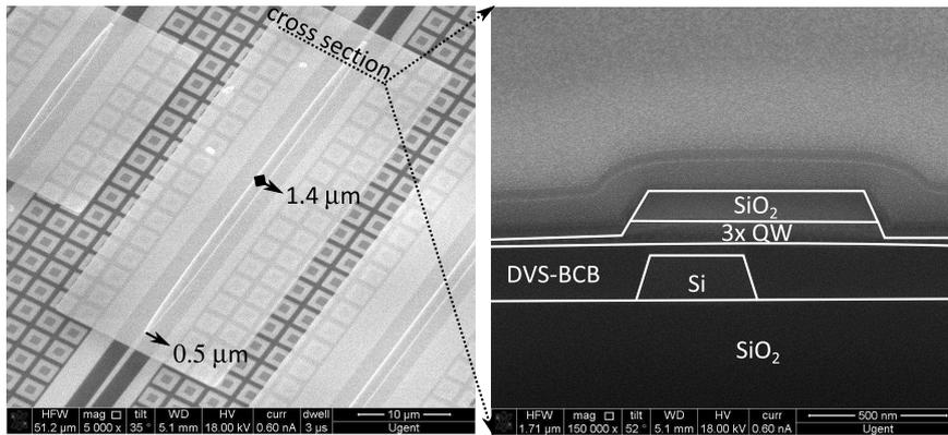
**Figure 3.24:** SEM micrograph of a device with cross section through the taper.
