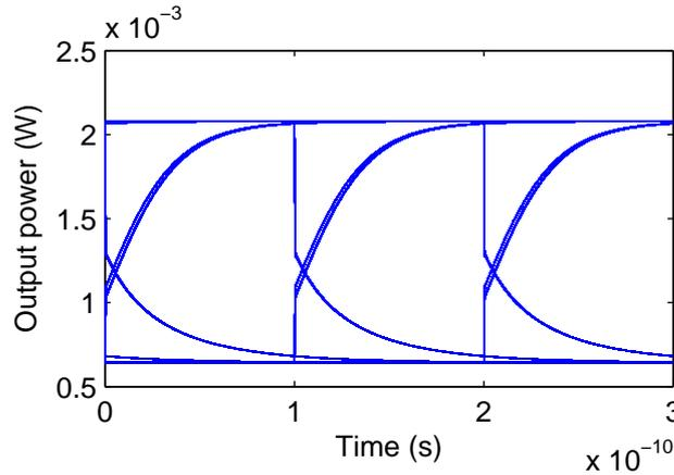
Figure 4.5: Simulated eye diagram at a bit rate of 10 Gbit/s.
