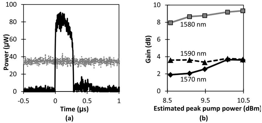
**Figure 3.23:** (a) Modulation in the probe signal (black) and reference trace (grey). (b) Net gain as a function of (estimated) pump pulse power.
