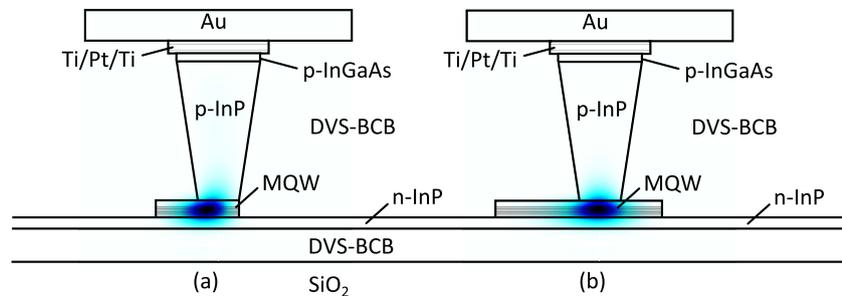
**Figure 2.26:** (a) p-waveguide of 1  $\mu\text{m}$  broad with 250 nm misalignment of active region to p-InP pillar position. (b) n-waveguide of 2  $\mu\text{m}$  broad with 250 nm misalignment of active region to p-InP pillar position.
