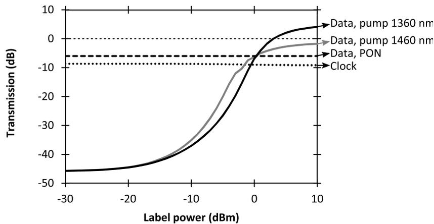
**Figure 5.27:** Simulation of the transmission through a 1x4 switch with state-of-the-art passives and well-passivated gates, both for pumping at 1460 nm and 1360 nm.
