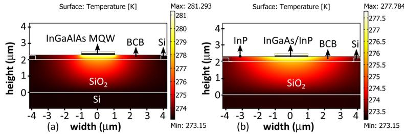
**Figure 3.5:** (a) Thermal profile for the stripe waveguide. (b) Thermal profile for the ridge waveguide.
