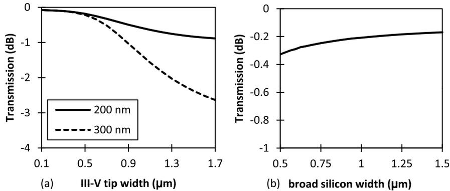
**Figure 2.17:** (a) Effect of the active region tip width on the device transmission of the fundamental TE-mode for a silicon width of  $1.25\ \mu\text{m}$ . (b) Effect of the width of the silicon wire underneath the III-V tip on the transmission of the fundamental TE-mode for a III-V tip of  $500\ \text{nm}$  wide.
