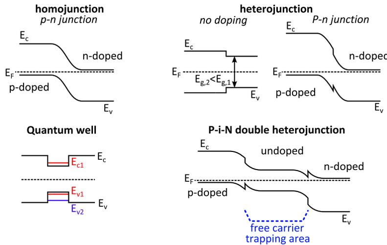
**Figure A.1:** Energy diagram of electrical confinement structures, showing conduction and valence band energies of the semiconductor materials.
