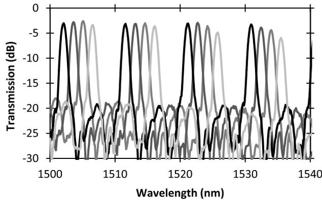
Figure 5.10: Transmission of the cyclic AWG design.
