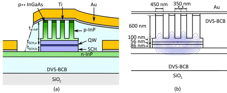
**Figure 2.2:** (a) Basic layout of the gallery waveguide structure used on the heterogeneously integrated III-V/SOI platform. (b) Mode profile in the optimized waveguide.
