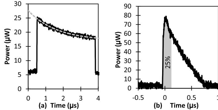
**Figure 3.22:** (a) Effect on the probe transmission of a 50 % duty cycle pump pulse train, with fitted exponential ( $\tau \approx 1.5 \mu\text{s}$ ). (b) Pump pulse shape used in the experiment. The gray area shows the time during which the corresponding probe modulation is averaged for calculation of the net gain.
