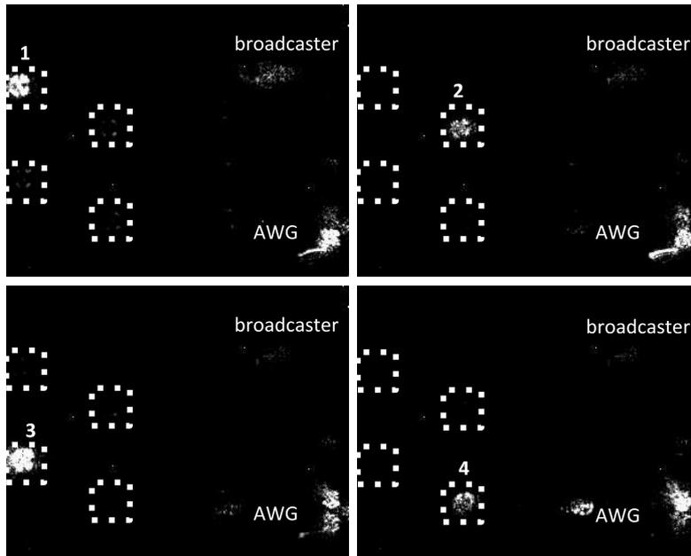
**Figure 5.22:** Static infrared images of label traversing the passives in the 1x4 switch. By changing the wavelength of the label, the label clearly ends up at the different MZI multiplexers at each output gate.
