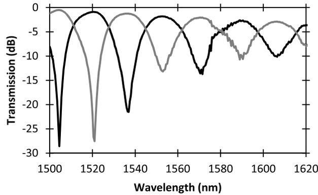
**Figure 5.8:** Transmission of the MZI design using a 10  $\mu\text{m}$  long directional coupler as 2x2 coupler.
