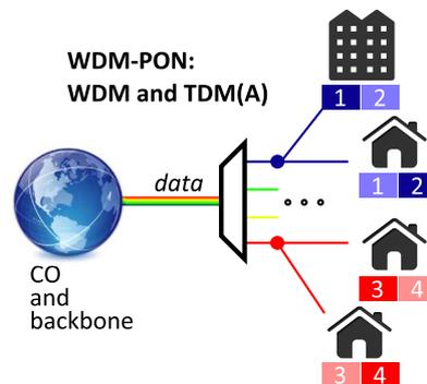
**Figure 5.2:** schematic of WDM-PON solution. Because of the WDM filtering the upstream data communication is more complicated, as the exact same wavelength needs to be used as for downstream communication.
