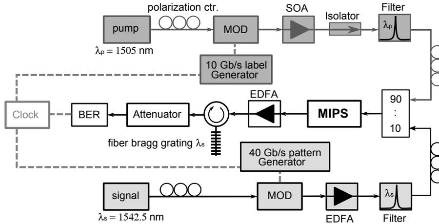
Figure 5.12: Setup for single gating experiment.
