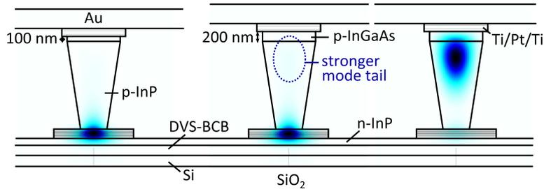
**Figure 2.14:** (left to right) Mode profile of fundamental TE mode in the unmatched case ( $t_{InGaAs} = 100$  nm,  $t_{SCH} = 32$  nm), fundamental TE mode in the matched case ( $t_{InGaAs} = 200$  nm,  $t_{SCH} = 32$  nm), and corresponding lossy mode with similar effective index.
