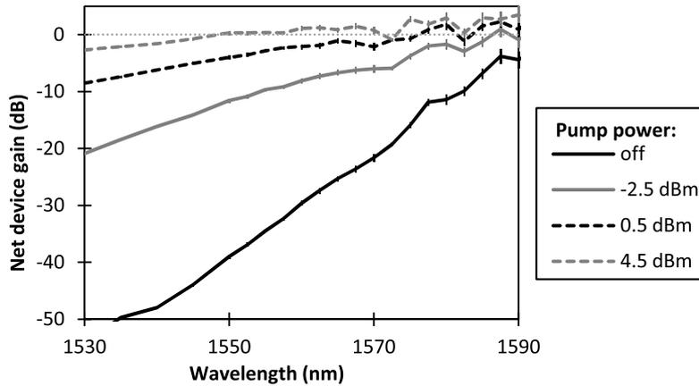
**Figure 3.25:** Probe transmission as a function of the probe wavelength, under different pumping conditions.
