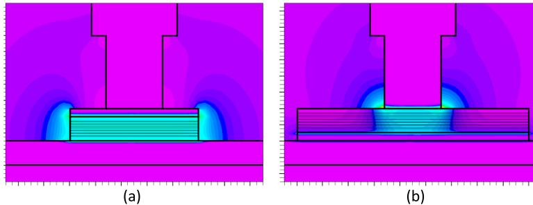
**Figure 2.20:** (a) Electric field distribution in the p-waveguide. (b) Electric field distribution in the n-waveguide.
