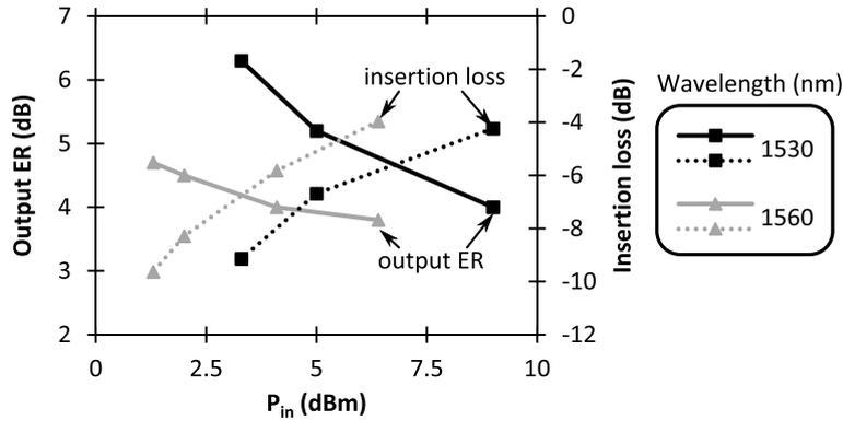
**Figure 4.14:** Insertion loss (dotted line) and output ER (solid line) as a function of input signal power for signals at 1530 nm and 1560 nm.
