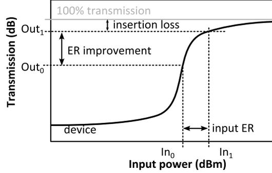
**Figure 4.1:** Regeneration concept: due to the non-linear transmission of the membrane device, the extinction ratio (ER) of the input signal can be improved.
