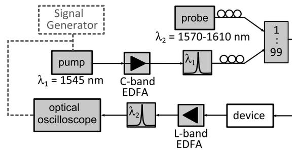
**Figure 3.21:** Setup of the pulsed experiment.
