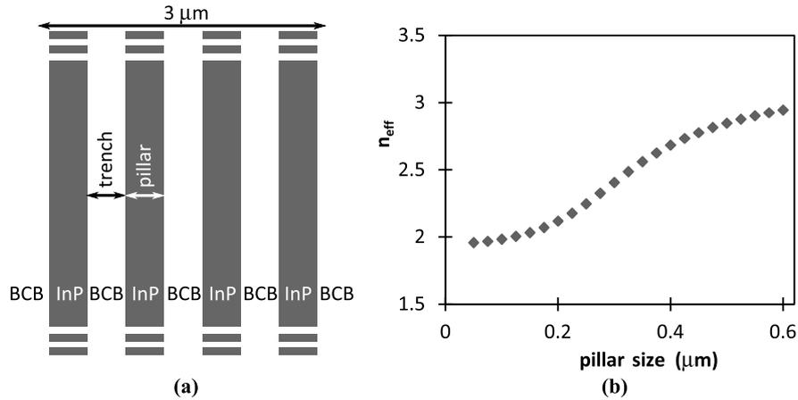
**Figure 2.3:** (a) Slab structure used to assess the effective index of the gallery layer. The number of pillars is always the maximal number that fits within 3 μm. (b) Effective index as a function of pillar width. The associated trenches have the same width as the pillars.
