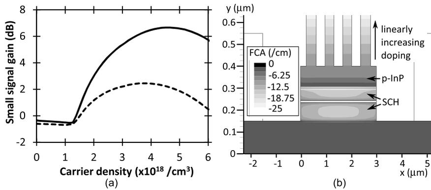
**Figure 2.10:** (a) Achieved small signal net gain as a function of the carrier concentration in the QW for the classical (dashed line) and gallery (solid line) design with a device length of  $200 \mu\text{m}$  long. The improved design of the gallery waveguide structure leads to a net gain that is two times higher than in the classical structure. (b) FCA in the gallery waveguide structure for an applied voltage of 1 V.
