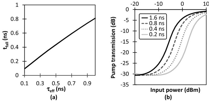
**Figure 3.12:** (a) Influence of  $\tau_{eff}$  on the device fall time  $t_{fall}$ . (b) Influence of  $\tau_{eff}$  on the pumping efficiency of the device.
