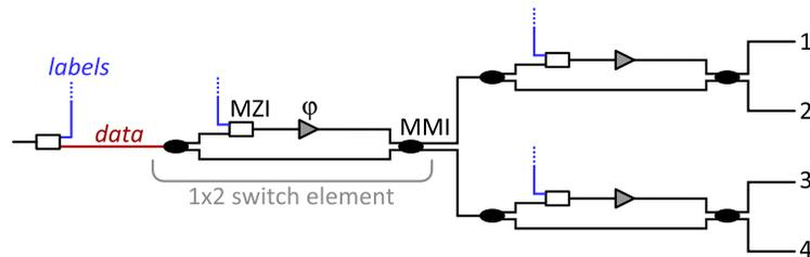
**Figure 5.5:** Schematic of implementation of concatenated MZI architecture using membrane gates as phase section. The MZIs in the variable phase arm are used to (de)multiplex the label and data wavelength bands.
