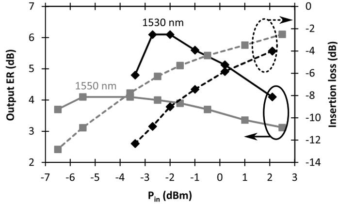
**Figure 4.10:** Insertion loss (dashed line) and output ER (solid line) as a function of input signal power for signals at 1530 nm and 1550 nm.
