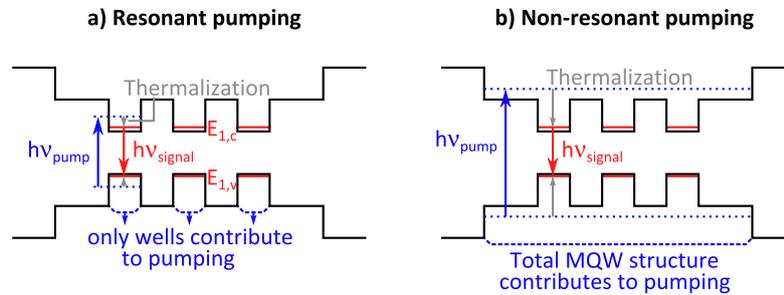
**Figure 3.2:** (a) Resonant optical pumping: only the QWs contribute. Note that the blue dotted line does not (necessarily) correspond to a higher QW level, but to a higher energy within the first QW level. (b) Non-resonant optical pumping: the total MQW structure contributes, however a lot of energy is lost as heat due to thermalization.
