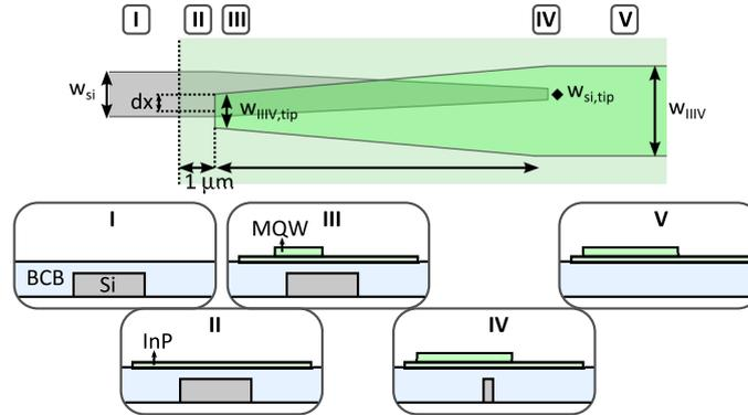
Figure 3.7: Schematic of the inverted taper coupler.
