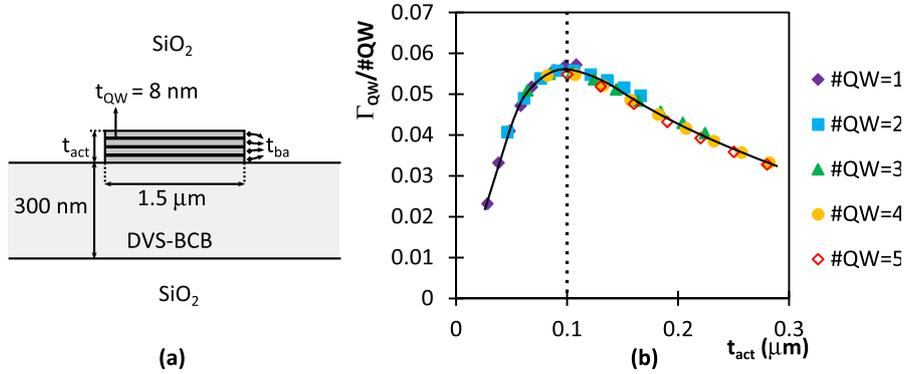
**Figure 3.1:** (a) Simulated waveguide structure: the barrier thickness  $t_{ba}$  as well as the number of QWs in the structure are parameters that are changed in the optimization procedure. The QW material is InGaAs, the barrier material is InP. (b) Confinement per QW.
