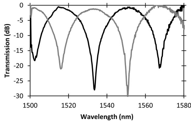
**Figure 5.9:** Transmission of the MZI design using improved MMI as 2x2 coupler.
