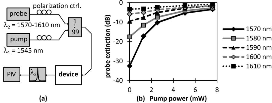
**Figure 3.20:** (a) Pump-probe setup. (b) Probe transmission as a function of pump power for different probe wavelengths.
