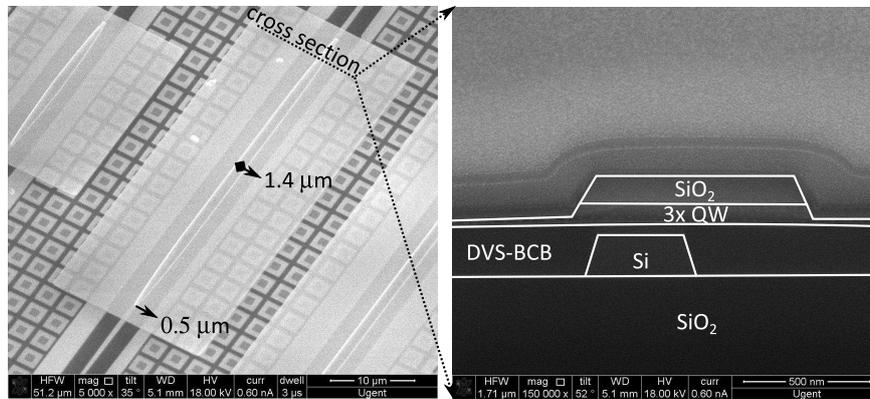
**Figure 5:** SEM micrograph of a membrane waveguide and cross section through the taper section.
