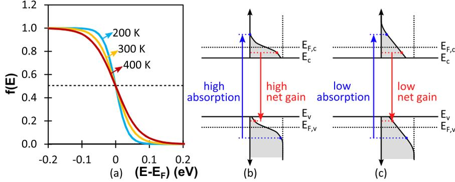
**Figure 3.3:** (a) The influence of temperature on Fermi-Dirac statistics. (b) Gain and absorption for at low temperatures with  $E_{F,c} > E_c$  and  $E_{F,v} < E_v$ . (c) Gain and absorption for high temperatures with  $E_{F,c} > E_c$  and  $E_{F,v} < E_v$ .
