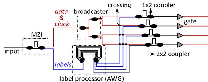
**Figure 5.7:** Detailed schematic of implementation of 1x4 broadcast-and-select switch using membrane gates.
