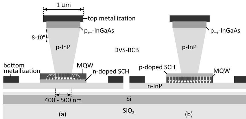
**Figure 2.13:** Basic layout of the V-waveguide structure optimized for modulator operation. (a) Without p-doped SCH layer, leading to a very low capacitance, but non-uniform electric field. Instead of a p-doped SCH layer, an n-doped SCH layer can be used in this case to achieve a certain active region thickness. (b) With p-doped SCH layer.
