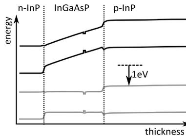
**Figure 2.6:** Band diagram at 0 V (top) and 1 V forward bias (bottom).
