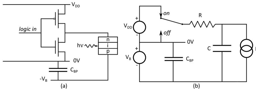
**Figure 2.12:** Based on [8] (a) Driving circuit for QCSE modulator. (b) Equivalent circuit.
