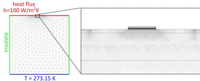
**Figure 3.4:** Mesh used for the thermal simulation of the membrane devices. Also the boundary conditions used in the simulation are shown.
