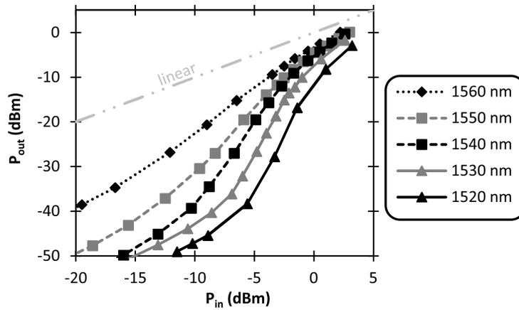
Figure 4.7: Static transmission through a 150  $\mu\text{m}$  long membrane.
