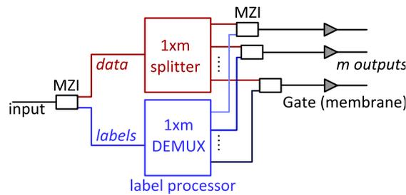
**Figure 5.4:** schematic of implementation of broadcast-and-select architecture using membrane gates. The MZIs are used to (de)multiplex the label and data wavelength bands.
