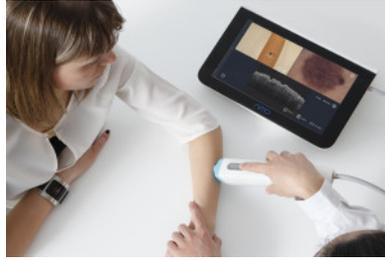
**Figure 1.12:** NITID, portable OCT imaging device for dermatology from DermaLumics. (image obtained from DermaLumics website [76])
