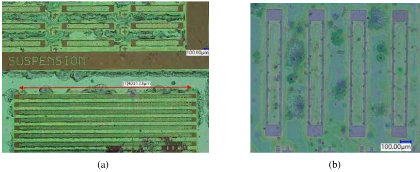
Figure 4.16: (a) Up to 4 mm long and 120 \mu\text{m} wide released PZT coupons with stress-release holes (b) up to 1 mm long and 120 \mu\text{m} wide suspended PZT coupons without holes.
