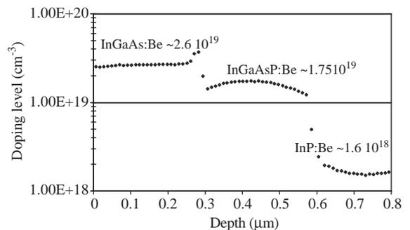
Fig. 2. ECV profile of an III–V hybrid contact comprising ternary and quaternary layers. The 300 nm-thick layers are used for an accurate p-type doping level measurement.
