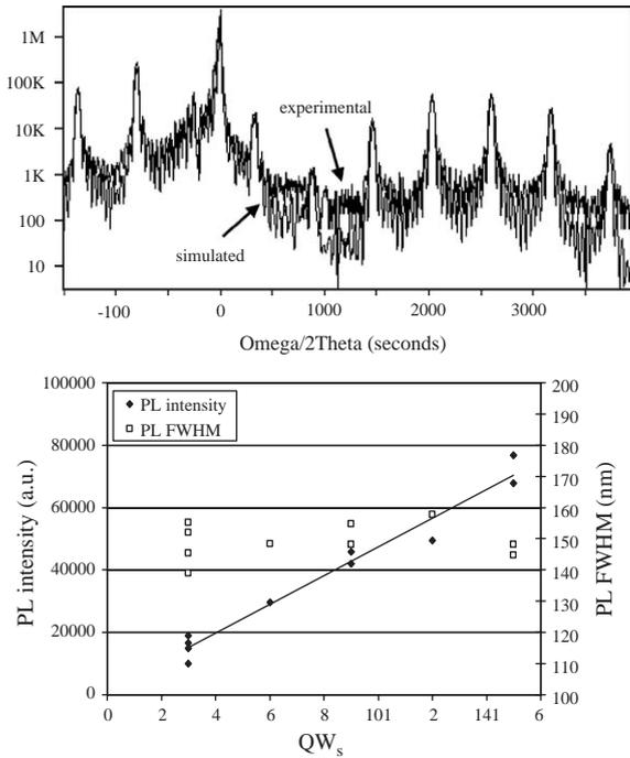
Fig. 3. Top: Experimental and simulated X-ray curves of a MQWs heterostructures comprising twelve  $-1.1\%$  tensile strained QWs. Bottom : Room temperature photoluminescence intensity and linewidth of  $-1.1\%$  tensile-strained MQWs as a function of QWs number.
