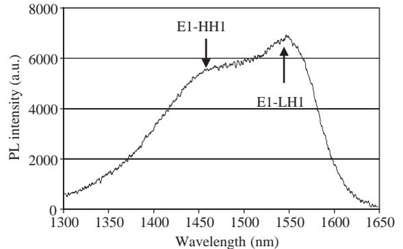
Fig. 6. Photoluminescence spectra of -1% tensile-strained MQWs showing electron/light-hole PL emission at 1.55  $\mu$ m.
