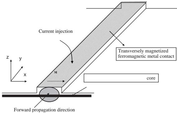
Fig. 1. Schematic illustration of the integrated optical waveguide isolator based on the dependence of the absorption coefficient on the propagation direction along the  $y$ -axis of the waveguide.
