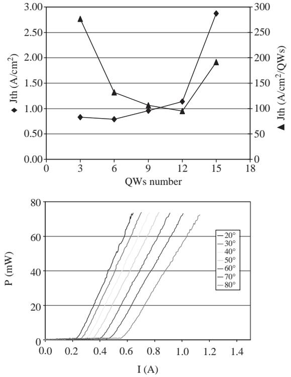
Fig. 5. Top: Threshold current density and threshold current density per QW of 600  $\mu$ m  $\times$  50  $\mu$ m BA lasers as a function of QWs number. Bottom : P(I) curves of a 600  $\mu$ m  $\times$  50  $\mu$ m BA laser for the 6 QWs heterostructure in the temperature range of 20–80 °C.
