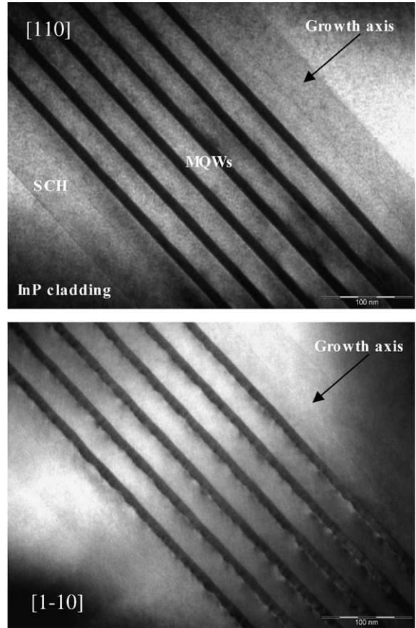
Fig. 4. [110] and  $[1\bar{1}0]$  cross-sectional TEM images of a six 12-nm-thick  $-1.1\%$  tensile-strained QWs heterostructures.
