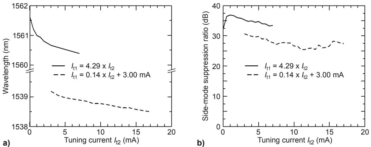
Fig. 9. Variation of emission wavelength (a) and SMSR (b) during continuous tuning (for two selected supermodes, shown as dashed lines in Fig. 7).
