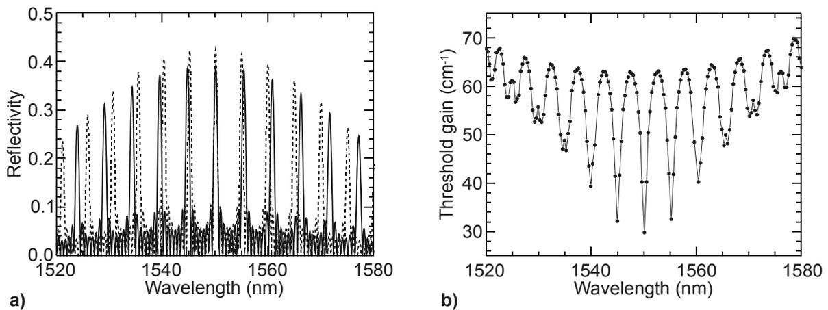
Fig. 2. a) Calculated reflection spectra of SGs with slightly different sampling periods. b) Cavity modes of the corresponding SG-TTG laser diode (dots indicate the position of the cavity modes, lines are only shown as a guide to the eye).
