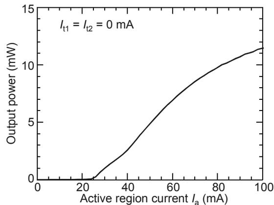
Fig. 6.  $L-I$  characteristics of an SG-TTG laser diode.
