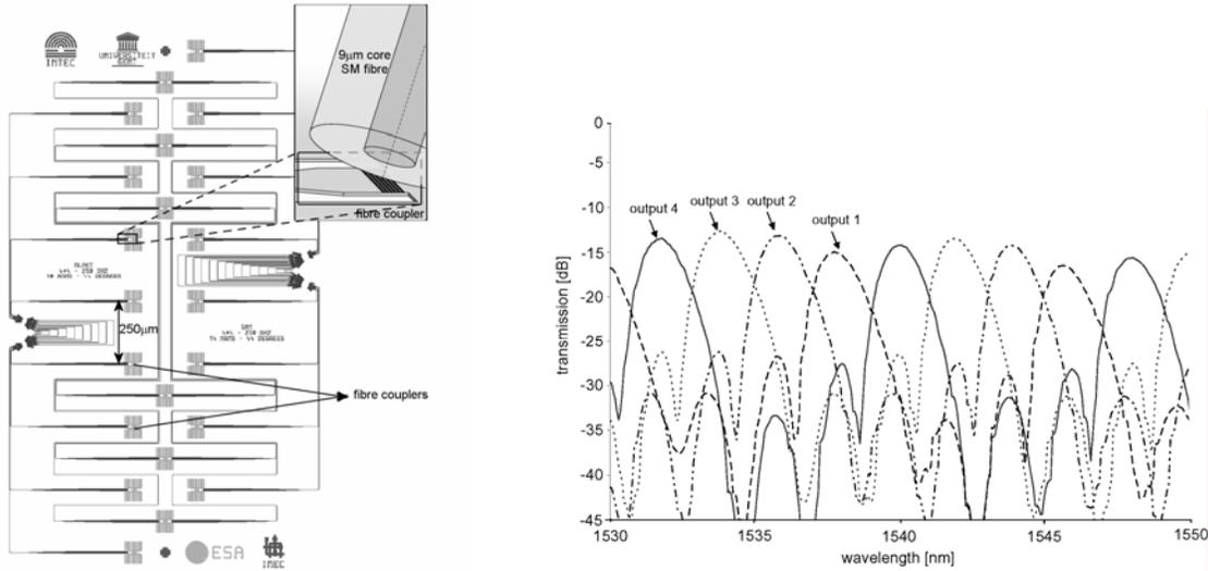
Fig. 1. (Left) Mask layout with AWG and fibre couplers. Spacing between the couplers is  $250\mu\text{m}$ , compatible with a standard array connector. (Right) Fibre to fibre transmission of the pigtailed device, from input 3 to all outputs
