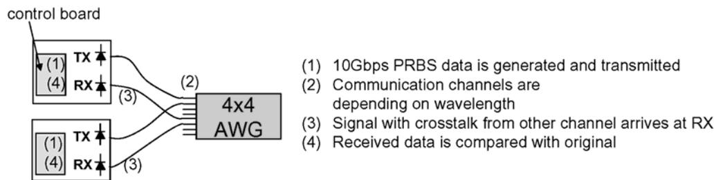
Fig. 2. Schematic of the high-speed wavelength-routed interconnect setup
