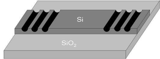
Fig. 1. Two identical fiber couplers fabricated with focused-ion-beam (FIB) on a  $10\mu\text{m}$  wide and 220nm thick Si waveguide.
