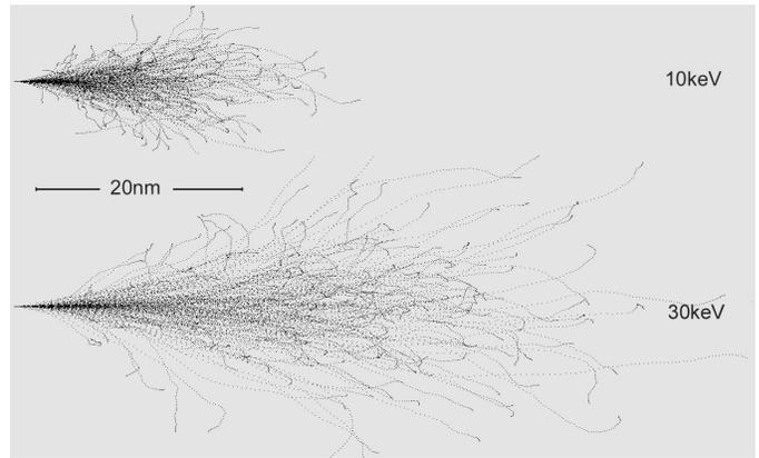
Fig. 3. Trajectories of 250 Ga ions accelerated to 10 and 30keV, perpendicularly projected on a Si target. Etching with 10keV ions produces a shallower damaged layer and less optical losses.
