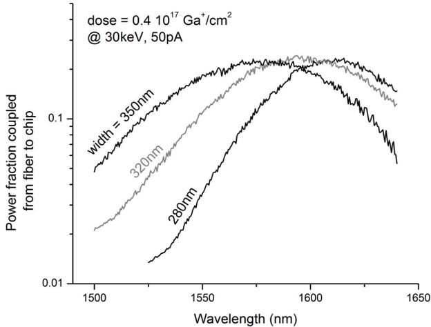
Fig. 5. The coupling efficiency of three gratings fabricated with  $I_2$  and  $Al_2O_3$ . The width of the scanned rectangles in the first etch step was varied from 280nm to 350nm to vary the central frequency.
