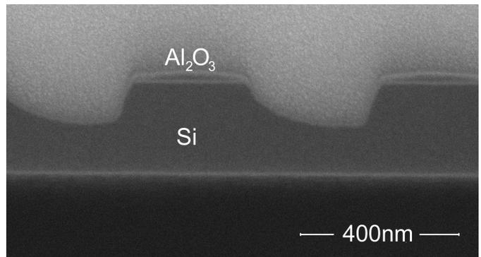
Fig. 4. Profile of a grating etched in Si with  $I_2$  as selective etch gas and  $Al_2O_3$  as hard mask. The profile is asymmetric due to the gas injection system.
