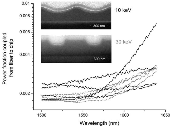
Fig. 2. Very inefficient fiber couplers fabricated directly into Si with 10keV (black) and 30keV (grey) Ga ions. The insets show the cross-sections through two grating periods: the 10keV beam is broader and makes a rounder profile, but still these gratings are the most efficient.
