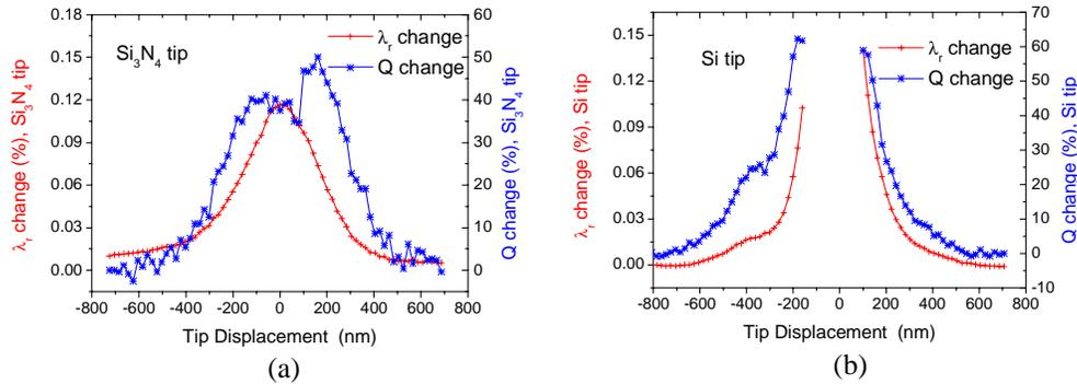
Fig. 5. Nano-mechanical tuning. (a) Change of  $Q$  and resonance wavelength detuning for a  $\text{Si}_3\text{N}_4$  probe versus  $y$ -displacement along the scan line shown in Fig. 4(a). (b) The same but now for a Si tip. In close proximity to the field maximum no data could be obtained because the transmission had dropped below the noise level.
