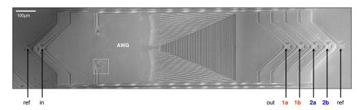
Fig. 6. SEM of fabricated duplexer. The outermost fiber couplers are directly connected and are used for as alignment and reference. The AWG has a  $600 \times 350 \, \mu m^2$  footprint. The two outputs for each wavelength band are not grouped but characterized individually.
