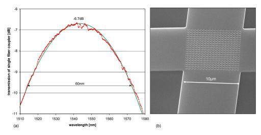
Fig. 7. 2-D grating fiber couplers: (a) Transmission of a single coupler, extracted from the transmission of the reference waveguide. (b) an SEM picture of the fiber coupler and access waveguides.
