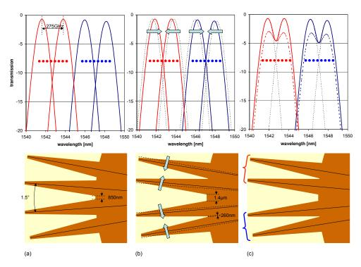
Fig. 4. Design of the AWG. (a) The transmission of the AWG output ports when located at their original channel spacings of 275 *GHz*. (b) The output ports are shifted towards each other in pairs. (c) When the signals in the ports are added up, two broad wavelength bands form. Full line: signals combined electrically (power); dashed line: signals combined using a lossless symmetric Y-junction.
