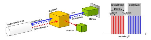
Fig. 1. Principle of duplexer-based fiber access end-point. The downstream and upstream operate each on one  $50\,GHz$ -spaced ITU channel within a  $400\,GHz$  band. By using a reflective approach, the channel can be selected at the central office.
