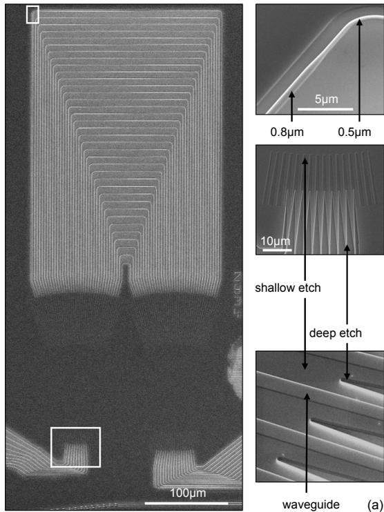
Fig. 1. Arrayed waveguide grating with  $16 \times 200GHz$  channels from [3]
