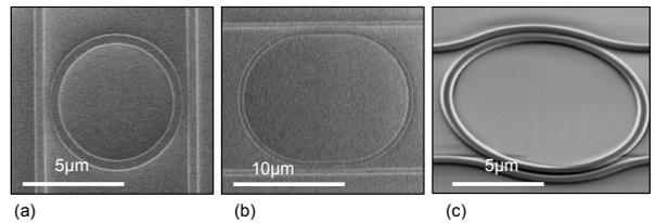
Fig. 4. Ring resonators from [2], [3], [6]. (a) Circular ring resonator,  $3\mu m$  bend radius; (c) racetrack resonator with a  $6\mu m$  bend and a  $3\mu m$  coupling section and (c) bend-coupled ring resonator with a  $5\mu m$  bend radius.
