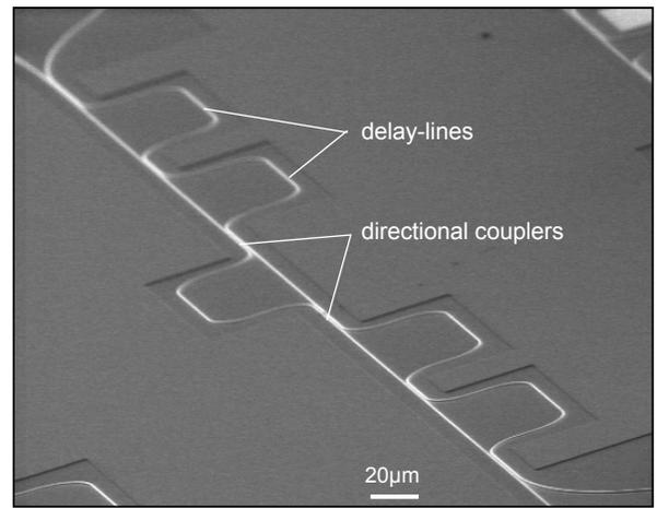
Fig. 3. A 5-stage Mach-Zehnder lattice filter from [3].
