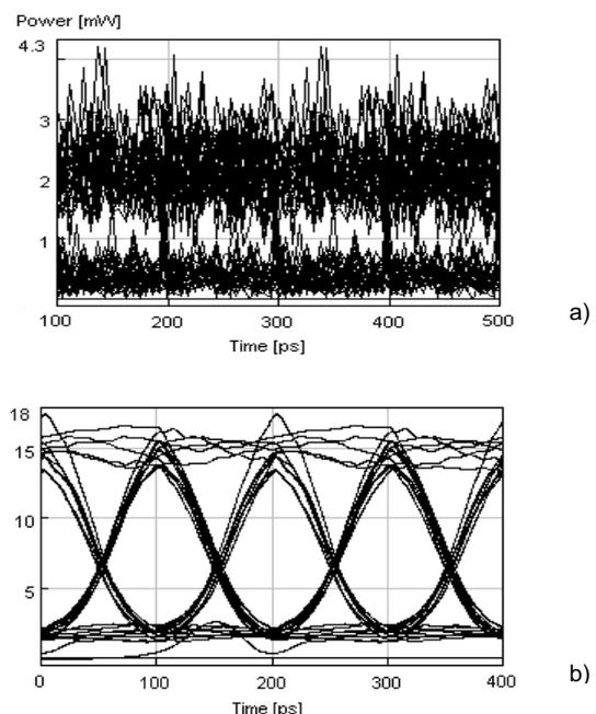
**Figure 2:** a) Eye diagram of a 10Gbit/s NRZ back to back signal with ER of 7.5dB. b) Eye diagram of the regenerated output signal with ER of 10 dB.
