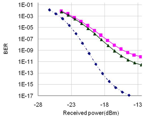
Figure 5 : BER as a function of the signal power incident on the receiver (dashed line is for the back to back signal and the others are for the wavelength converted laser output signal (triangles are for  $dg/dN = 6 \cdot 10^{-20} \text{ m}^2$  and squares are for  $dg/dN = 5 \cdot 10^{-20} \text{ m}^2$ ).
