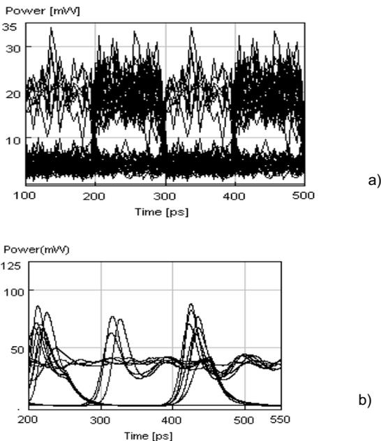
Figure 4: a) Eye diagram of a 10Gbit/s NRZ back to back signal with ER of 6.5dB. b) Eye diagram of the output signal after passage through the device with ER of 18 dB.
