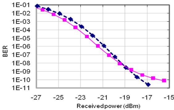
Figure 3 : BER as a function of the signal power incident on the receiver (dashed line is for the back to back signal and solid line is for regenerated output signal).
