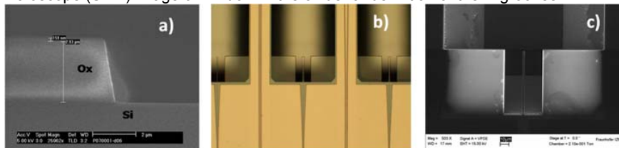
Figure 2: a) Edge of window in the oxide for definition of the V-grooves. b) Optical microscope and c) SEM images of fabricated samples.
