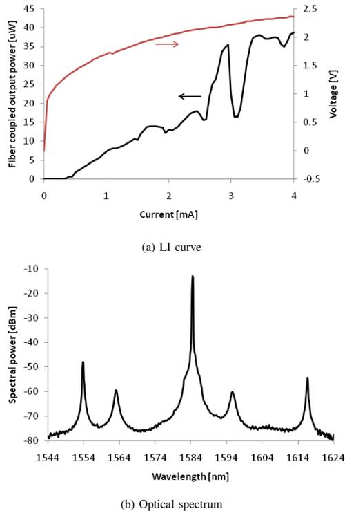
Fig. 3. LI curve (a) and spectrum (b) of a 7.5  $\mu\text{m}$  diameter microdisk
