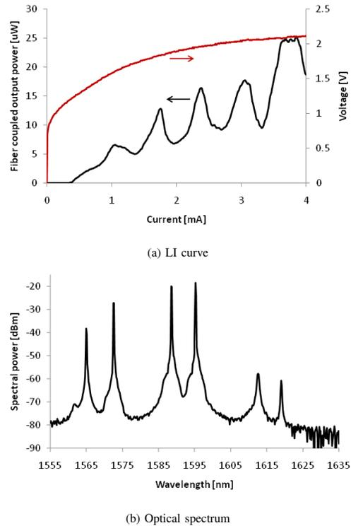
Fig. 4. LI curve (a) and spectrum (b) of a 10  $\mu\text{m}$  diameter microdisk
