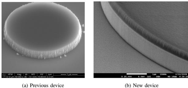
Fig. 2. SEM pictures of the previous device (a), and the new device with reduced sidewall roughness (b).
