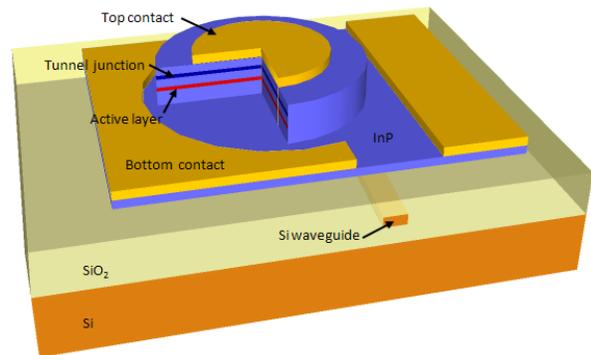
Fig. 1. Schematic representation of a heterogeneously integrated microdisk laser on SOI.
