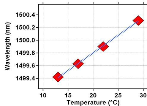
**Fig. 3:** Wavelength versus temperature of the sample in low duty-cycle regime.
