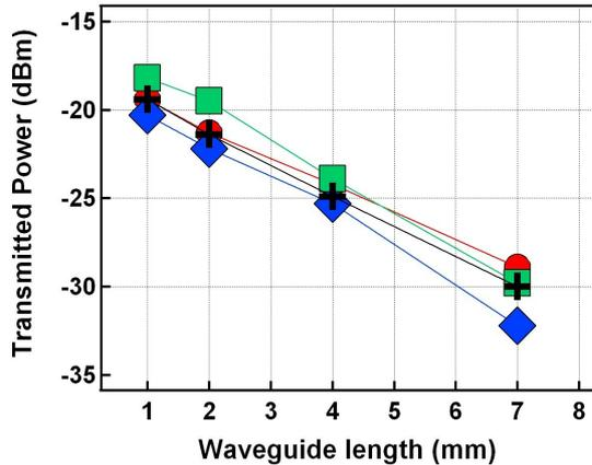
**Fig. 2:** Transmitted power (in dBm) versus waveguide length for different DN concentration: 0 % (circles), 2.5 % (cross), 5 % (diamond shape), 10 % (square)
