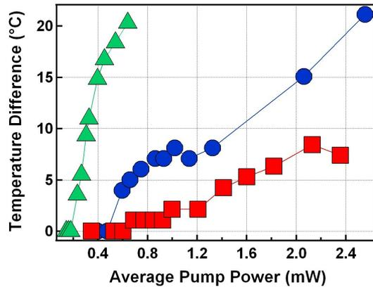
**Fig. 3:** Temperature difference versus average pump power at 7,5 % duty cycle (30ns pulse) for 0% (triangle), 5 % (circle), 10 % (square)
