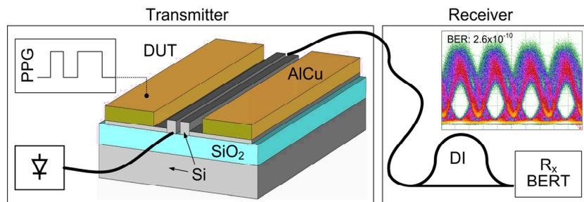
**Figure 3:** Data transmission experiment: Laser light is launched into the SOH slot waveguide, and an electrical 42.7 Gbit/s signal is fed to the electrodes. This generates a purely phase-modulated signal. On the receiver side, phase-to-amplitude conversion is achieved by feeding the signal into a delay interferometer (DI) that superimposes optical waves from subsequent bit slots. DUT = device under test, BERT = bit-error ratio tester
