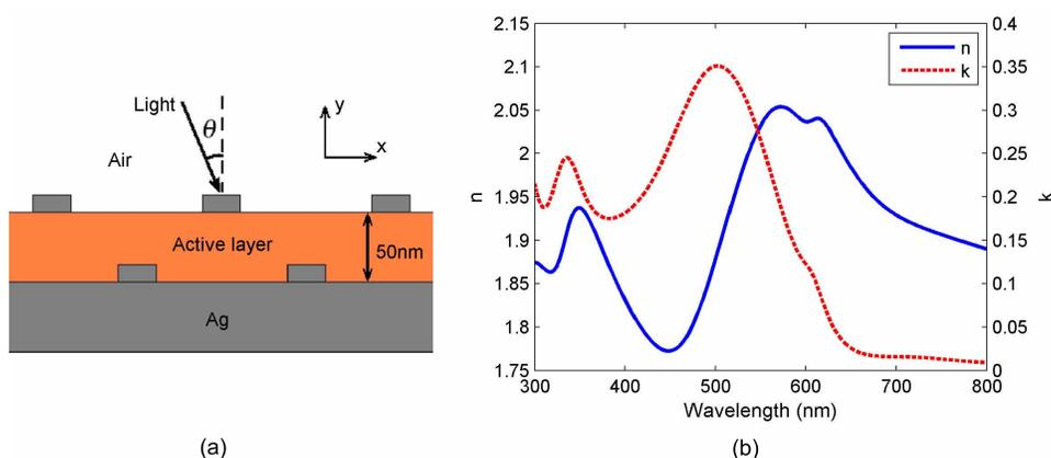
Fig. 1. (a) Schematic diagram of OSCs with combined gratings (front and back grating). (b) Optical constants of P3HT:PCBM with 1:1 weight ratio,  $n$  and  $k$  are the real and the imaginary parts of the refractive index.
