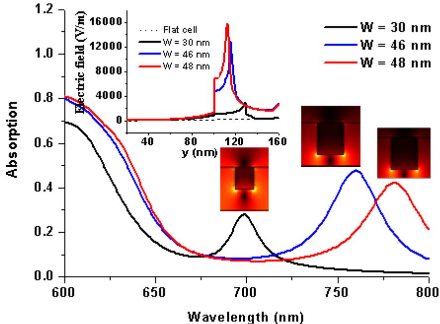
Fig. 6. Absorption in active layer for various sizes of Ag square grating (the absorption profiles corresponding to the absorption peaks are shown above the peaks). The inset is a cross-section of the field along the edge of the grating, from air to the active layer side.
