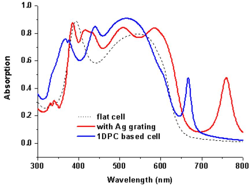
Fig. 4. Absorption in the active layer for the bare OSC (dotted line), the cell with Ag square grating (red solid line), and 1D PC (blue solid line).
