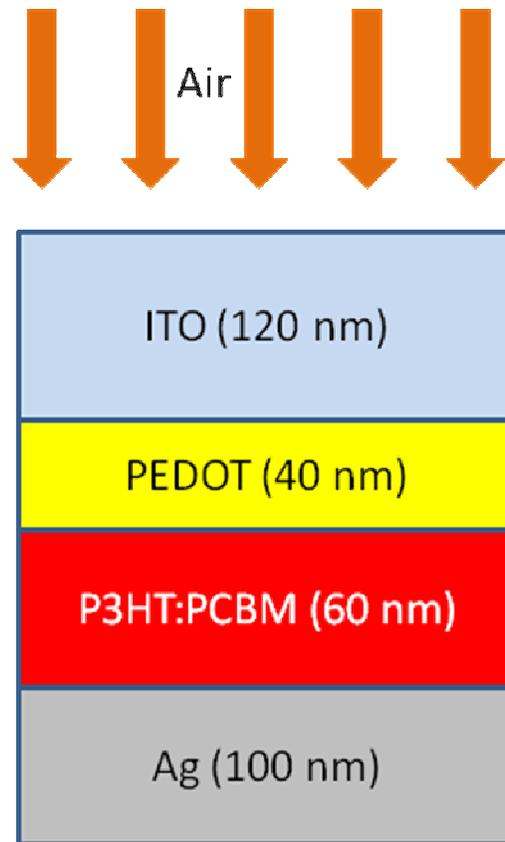
Fig. 1. Cross-section of the reference flat OSC.
