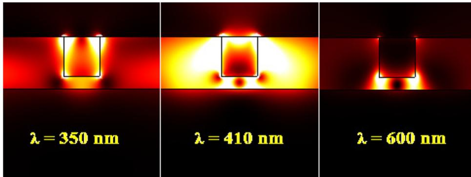
Fig. 5. Absorption profiles of OSCs with optimal Ag square grating with  $W = 46$  nm and  $P = 350$  nm at various wavelengths ( $\lambda$ ).
