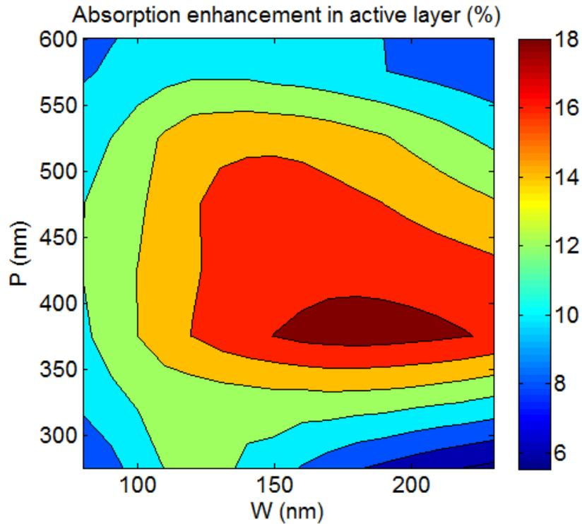
Fig. 8. Absorption enhancement in the active layer varying the ITO width (W) and periodicity (P).
