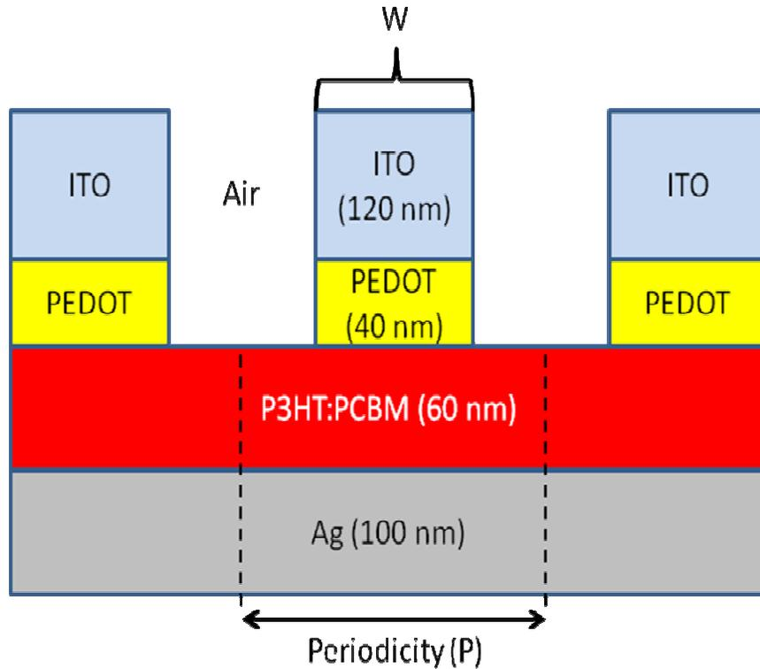
Fig. 7. Cross-section of OSC with 1D photonic crystal patterned on top.
