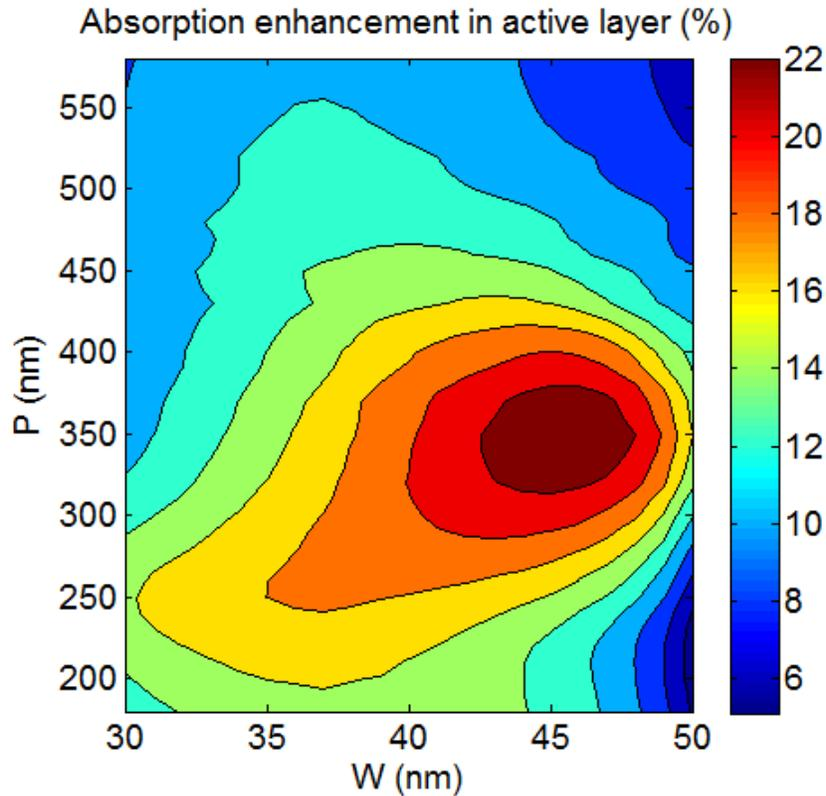
Fig. 3. Absorption enhancement in active layer for various sizes of Ag square grating with width (W) and periodicity (P).
