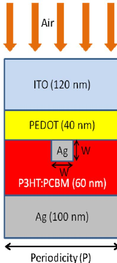
Fig. 2. Cross-section of OSC with Ag square grating integrated inside the active layer.
