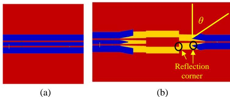
Figure 3. (a) A reference design with suppressed reflections. (b) A design with the deeply etched walls titled angle  $\theta$ .
