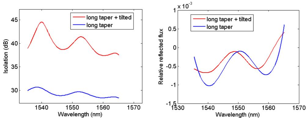
Figure 5. Isolation and relative reflection of MMIs with longer tapers. The blue curve is an MMI with the deeply etched walls tilted by  $60^\circ$ , and moved  $8\ \mu\text{m}$  away from the MMI core using a longer taper. The red curve has the same deeply etched walls, but has its MMI core walls also tilted outward by  $20^\circ$ .
