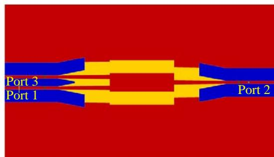
Figure 1. A commonly used 2x1 MMI on SOI. In the red area, a silicon layer with a thickness of 220 nm is covered on top of the silica buffer layer. In the yellow area the silicon is etched down to 150 nm. The silicon layer is etched away in the blue area, and this area is used as the trench for wire waveguides.
