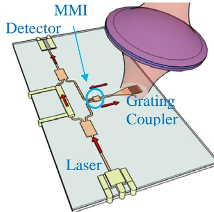
Figure 2. Schematic show of an on-chip LDV with an MMI as the splitter.
