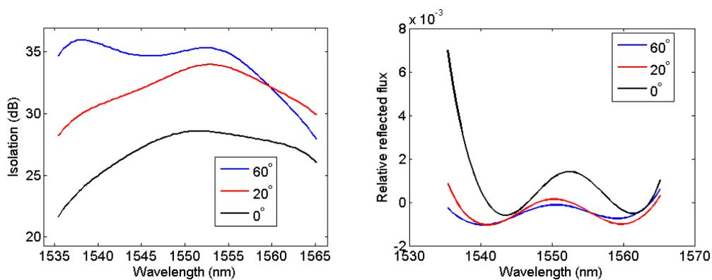
Figure 4. Isolation and relative reflection of MMIs with different tilting angles of the deeply etched walls.
