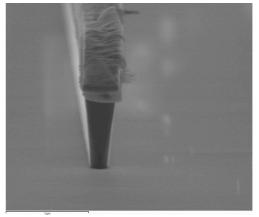
Figure 2 Cross-section of fabricated taper tip
