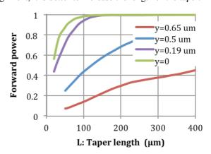
Figure 3 Simulation of power transmitted through tapered transition as function of taper length, and for different values of misalignment (500nm taper tip, 80nm bonding layer thickness).
