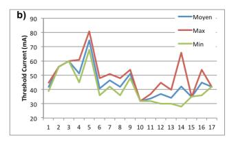
Figure 5 a) Maximum output power and b) threshold current for different laser designs. The horizontal axis denotes the design number. Red/Blue/Green denote maximum/average/minimum values over 5 identical devices per laser design.
