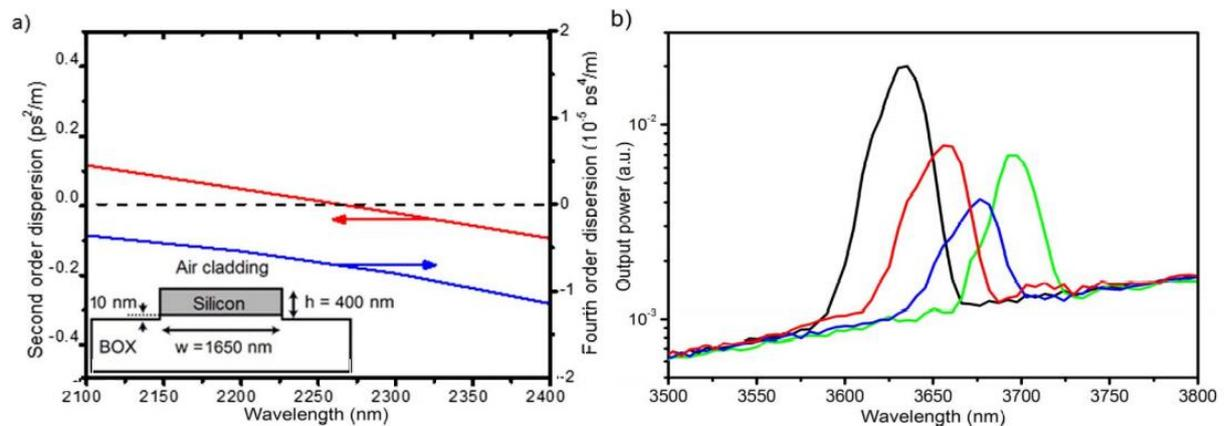
Figure 1: a) The dispersion of the silicon waveguide shown in the inset. B) the downconverted signals of respectively a telecom signal at 1565 nm (black), 1559 nm (red), 1554 nm (blue), and 1550 nm (green).
