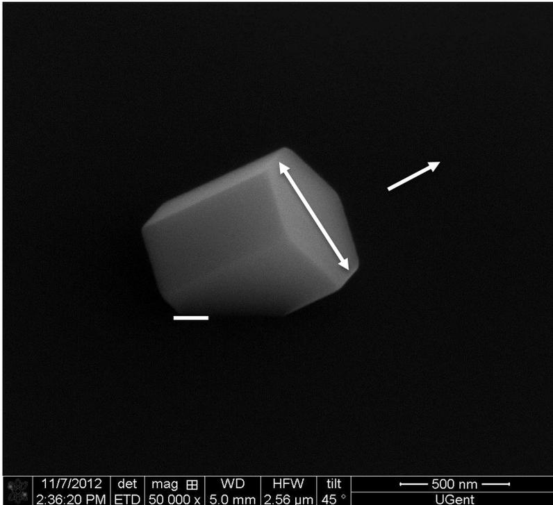
1. Nanowires of more than 500 nm diameter grown on top of InP island of below 100 nm diameter. The length is about 1 μm.
