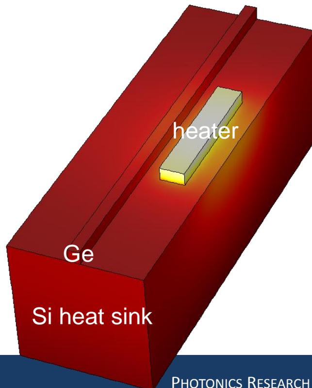
350mW power consumption for  $\pi$  phase shift
