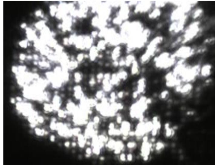
35 nano-lasers are successfully fabricated out of 80 sites.
