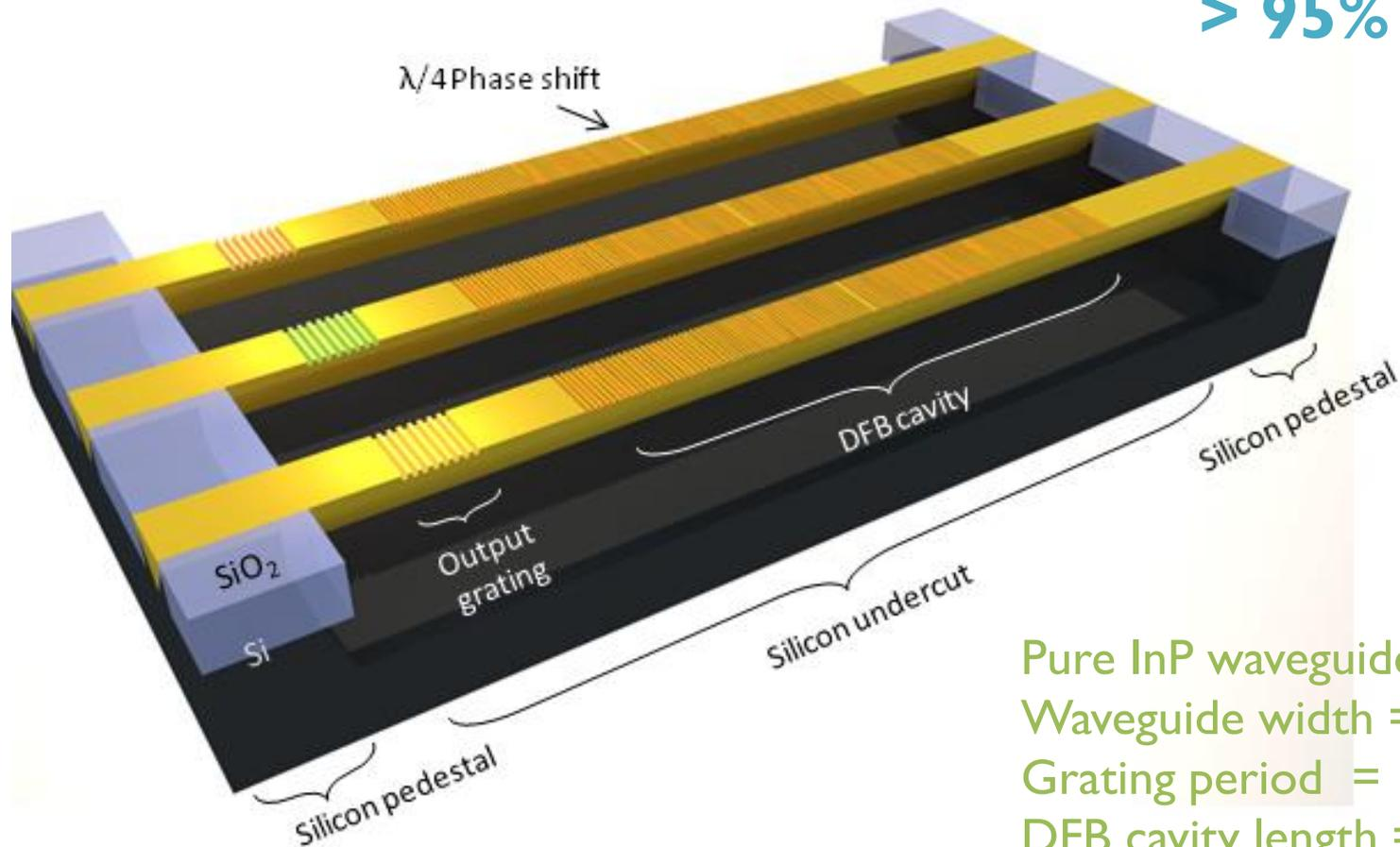
Pure InP waveguide
