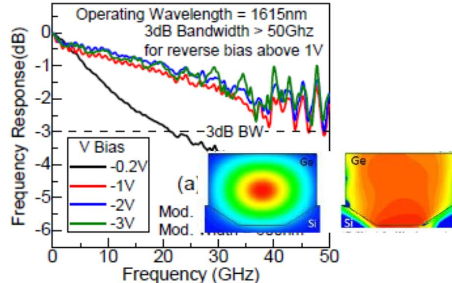
strong confinement of optical and electrical field enabled by submicron Ge/Si waveguide platform
