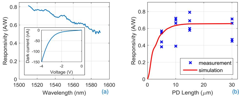
Fig. 3. (a) Responsivity versus wavelength of a  $3 \times 10 \mu\text{m}^2$  UTC-PD measured at  $-4 \text{ V}$ ; the inset shows the measured dark current versus bias voltage. (b) Responsivity as a function of the length of the UTC-PDs. Both measurement data and simulation results are shown.
