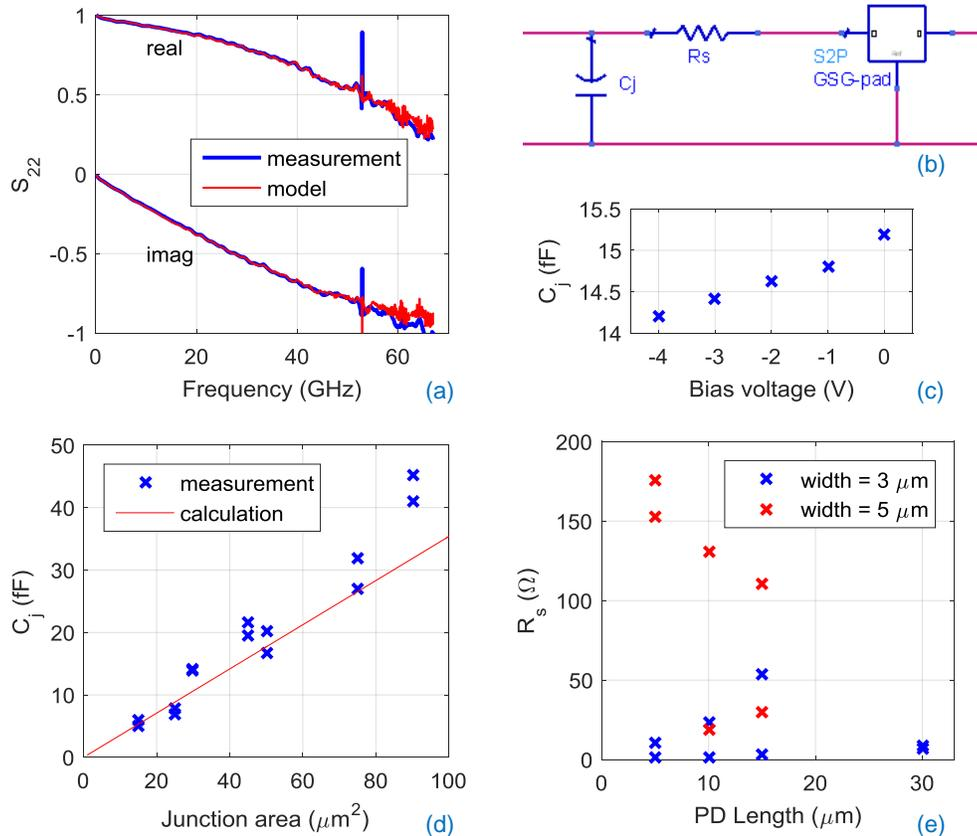
Fig. 6. (a) Real part and imaginary part of the reflection coefficient ( $S_{22}$ ) of a  $3 \times 10 \mu\text{m}^2$  UTC-PD. Results from measurements and modeling are both shown. (b) The equivalent circuit model of the UTC-PD. (c) Bias dependence of the junction capacitance ( $C_j$ ) extracted from the model. (d)  $C_j$  of different UTC-PDs as a function of the junction area. (e) Series resistance ( $R_s$ ) of different UTC-PDs versus their length.
