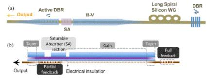
Figure 1: Layout of the III-V-on-silicon mode-locked laser cavity: (a) top view; (b) longitudinal cross-section.
