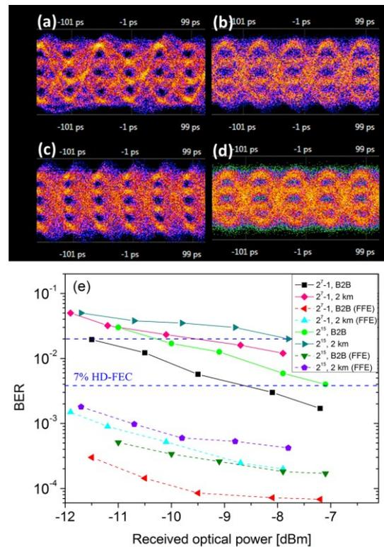
**Fig. 3:** Eye diagrams for PAM-4 at 20 GBaud in back-to-back configuration and after 2km of transmission over NZ-DSF for a PRBS length of 2<sup>7</sup>-1 (a,b) and for a length of 2<sup>15</sup> (c,d). BER measurements for back-to-back and 2 km NZ-DSF configuration (bottom).
