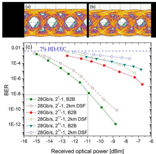
**Fig. 2:** Eye diagrams for back-to-back (a) and after 2 km NZ-DSF fiber transmission (b) at 28 Gb/s using a 2<sup>11</sup>-1 data pattern length (bias current of 100 mA at 20 °C), BER curves for different PRBS pattern lengths (c).
