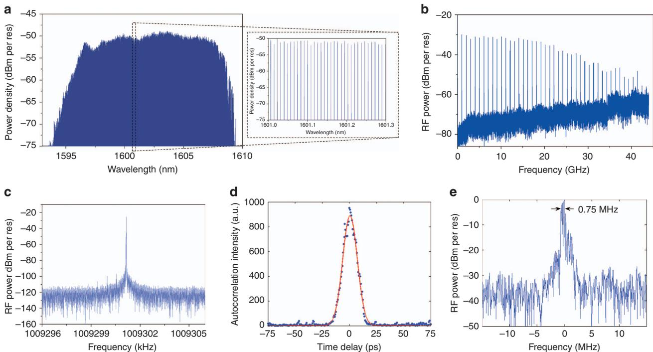
**Figure 6** (a) High-resolution optical spectrum of the optical comb when the MLL is hybrid mode-locked (inset: magnification of the optical spectrum). (b) RF spectrum of the generated pulse train. (c) Fundamental RF peak over a span of 10 kHz. (d) An auto-correlation trace of the output pulse when the laser is hybrid mode-locked. (e) Beat note between the optical comb and the tunable laser at a wavelength of 1607 nm, which indicates that the linewidth of the optical mode is smaller than 1 MHz.
