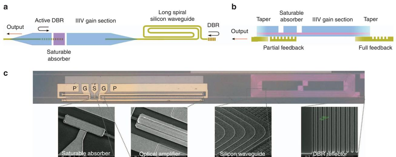
**Figure 1** (a) Top and (b) side views of the anti-colliding MLL design. (c) Microscope image of the III-V-on-Si MLL. Insets: Scanning electron microscope images of various constituent parts of the laser.
