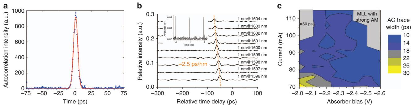
**Figure 5** (a) An auto-correlation trace and the corresponding fit of the MLL output. (b) The recorded pulse traces by a real-time oscilloscope for different parts of the optical comb. The inset shows a time trace of the pulse trains, which were recorded using a real-time oscilloscope. (c) Mapping of the auto-correlation trace width over the current injection and SA bias. The arrow indicates the optimal operation point.
