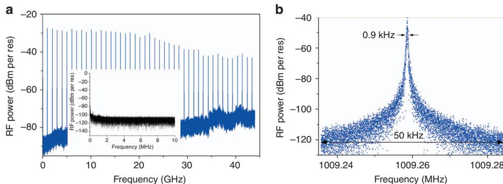
**Figure 3** (a) RF spectrum of the generated pulse train (RBW 300 KHz, VBW 10 KHz) when the laser is operated at the optimal operation point of Figure 2c. Inset: enlarged RF spectrum in the frequency range of 1–10 MHz (b) Detail of the 1-GHz RF tone (RBW 10 Hz, VBW 10 kHz).
