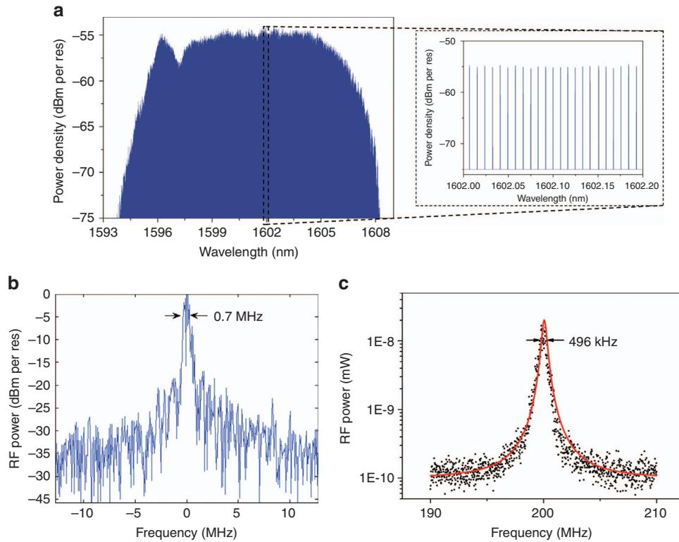
**Figure 4** (a) An optical comb generated by the passively locked 1 GHz MLL. Inset: a detail of evenly spaced optical modes in the comb. (b) Beat note between the optical comb and the tunable laser at a wavelength of 1600 nm. (c) Measured optical linewidth of the MLL using the delayed self-heterodyne method, which indicates an optical linewidth below 250 kHz. The black dots are the measured data, and the red curve is the corresponding Lorentzian fitting.
