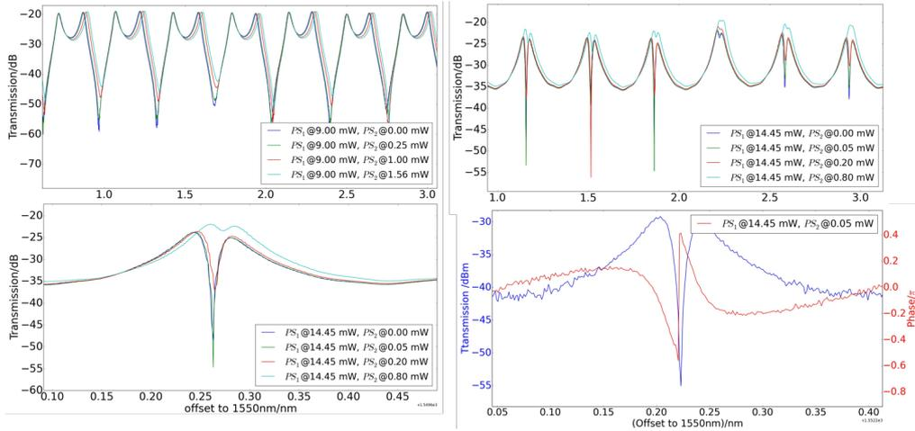
Figure 5: (a) shows the generation of Fano resonance if the FP mode and ring resonance are not perfectly aligned. (b) gives the transition from Fano resonance to EIT when precisely tune the FP mode to make it aligned with ring resonance. (c) provides a zoomed view of one resonance. (d) shows the phase response of such a EIT peak.
