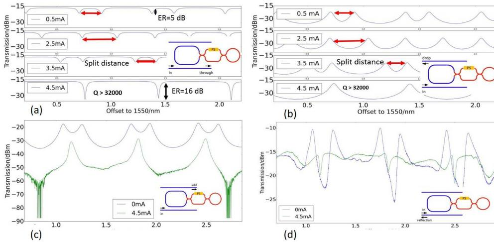
Figure 3: (a) demonstrates the splitting elimination in the *through* port (b) shows the same compensation for the output at the *drop* port, while (c) and (d) show how our device can suppress the unwanted output from *add* and *in* port.
