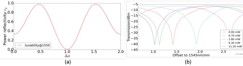
Figure 2: Simulation shows that  $\frac{\pi}{2}$  radians added to the phase shifter can generate a reflectivity change from 0 to 100% (a). Measurement proved 6 mW would lead to a 35 dB change in its reflectivity (b).
