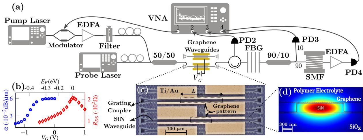
Fig. 1: (a) Setup for the XAM/XPM experiment. (b) Waveguide loss (blue) and the electrical resistance over the graphene (red) as function of  $V_G$ . (c) Top-view of the sample. (d) Cross-section of a SiN waveguide with TE<sub>00</sub> mode.
