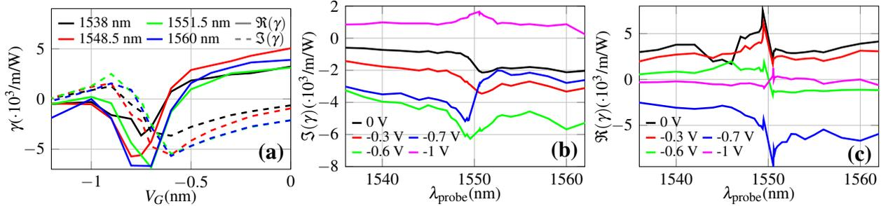
Fig. 2: Experimental results. The waveguide width and height are respectively 1400 nm and 330 nm, the graphene length 50  $\mu\text{m}$ ,  $\lambda_{\text{pump}}=1550.18$  nm. (a)  $\Re\gamma$  (solid) and  $\Im\gamma$  (dashed) as a function of  $V_G$ , for different values of  $\lambda_{\text{probe}}$  (see legend). (b, c)  $\Im\gamma$  and  $\Re\gamma$  as a function of  $\lambda_{\text{probe}}$ , for different values of  $V_G$  (see legend).
