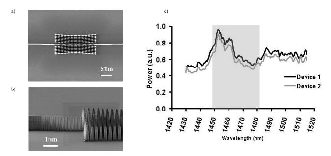
Fig. 3. (a) Top-down SEM image of tapered photonic crystal waveguide (b) Side view SEM of tapered photonic crystal waveguide (c) transmission measurement through the structures in (a) and (b). Two PC waveguides fabricated on the same chip demonstrated similar transmission.
