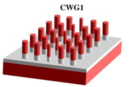
Fig. 1. Schematic representation of a 2D slab photonic crystal waveguide made of cylindrical dielectric pillars.
