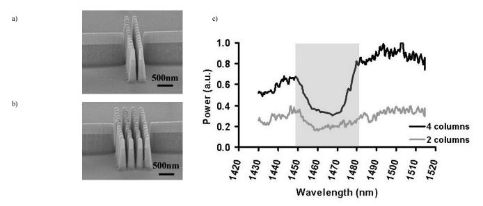
Fig. 2. (a) Scanning Electron Microscope (SEM) image of photonic crystal with 2 columns of dielectric pillars (b) SEM of a photonic crystal with 4 columns of dielectric pillars (c) transmission measurement through the structures in (a) and (b).
