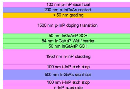
Fig. 5. Schematic of the epi layer stack.
