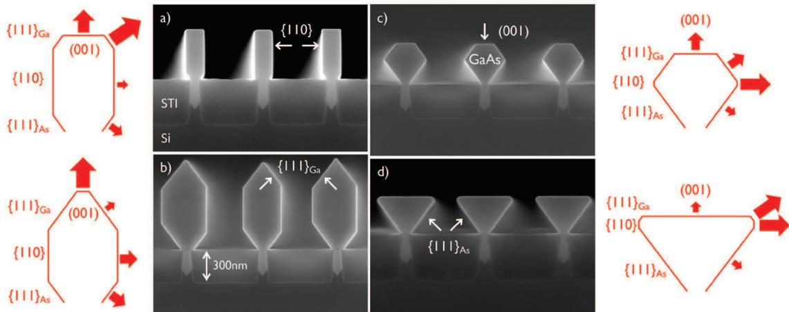
Cross-section scanning electron microscopy images of GaAs nano-ridges deposited under different MOCVD growth conditions and the corresponding sketch to indicate the different growth rate hierarchies. The size of each red arrow indicates the growth rate on the particular facets (the bigger the arrow, the higher the GaAs growth rate).
