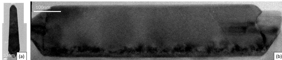
Figure 5. (a) Perpendicular and (b) parallel view TEM analysis of the InP/Si heterostructure grown in “V-grooved” for a 20-nm-width trench
