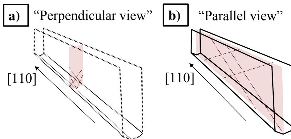
Figure 2. III-V selective area growth on Si(001) in trenches. (a) “*Perpendicular view*” presenting an efficient trapping effect of (111)-oriented defects from the III-V/Si interface. (b) “*Parallel view*” where (111)-oriented defects are not trapped in the direction along the trench.
