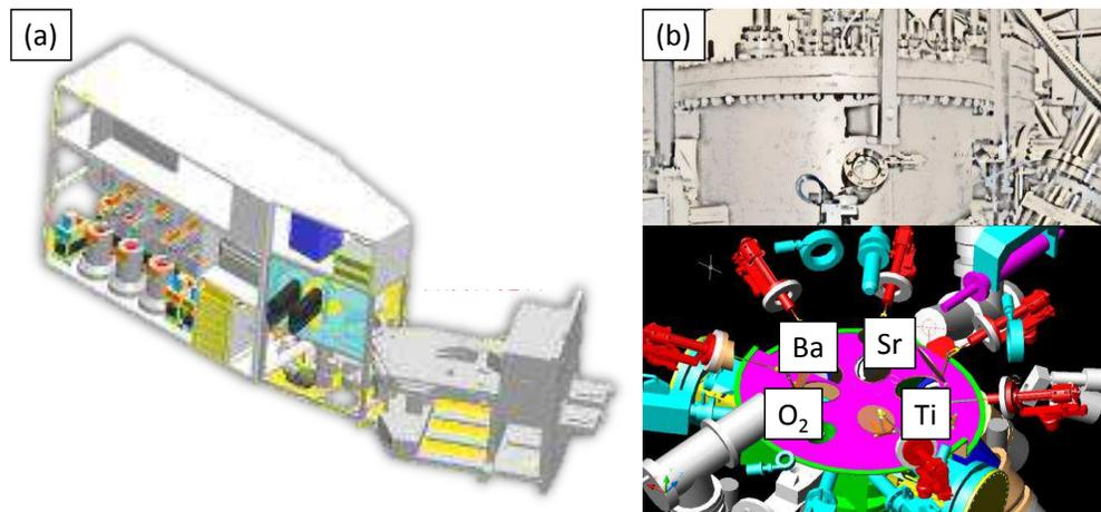
Figure 1. (a) Schematic of the 300mm MOVPE tool installed in imec clean room used for the III-V selective area growth.(b)Schematic of the 200mm MBE oxide reactor with the different sources used for epitaxial oxide growth.
