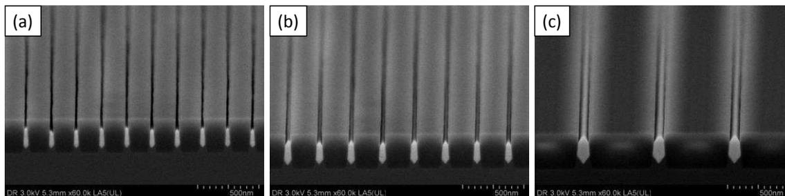
Figure 3. Tilted view SEM images after InP heteroepitaxy on patterned Si(001) in (a) 20nm, (b) 40nm, (c) 100nm widths trenches.
