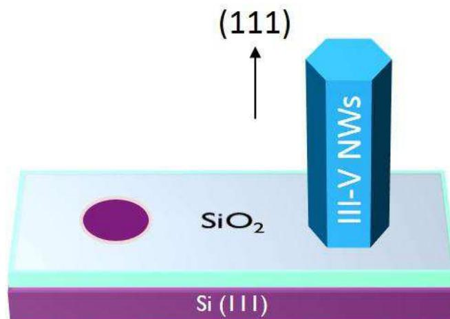
Figure 6. Schematic of selective area growth of III-V NWs on Si(111) from holes in oxide template.
