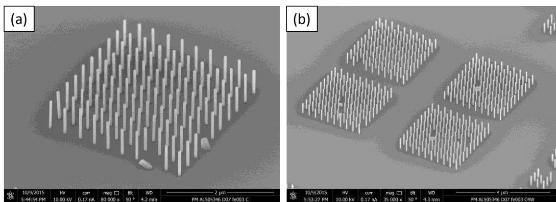
Figure 7. SEM images of  $\text{In}_{0.5}\text{Ga}_{0.5}\text{As}$  NWs in (a)  $D=60\text{nm}$  contact area and (b)  $D=30\text{nm}$  device area.
