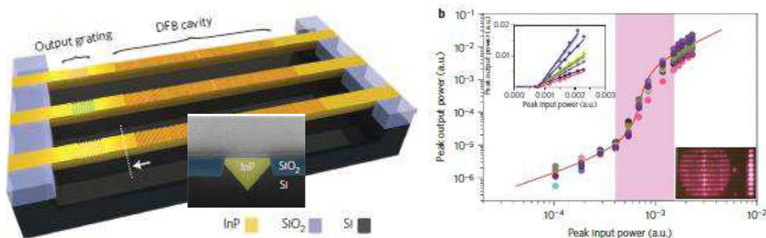
Figure 8. (a) Schematic plot of the InP DFB laser array integrated on silicon. Insert: SEM image of a InP-on-Si waveguide (b) Measured L-L curves of an array of ten DFB lasers. Inset: linear-scale version of the ten log-scale L-L curves presented in the main panel. Inset (bottom): camera-recorded photoluminescence image of ten working lasers under a large-area pumping condition.
