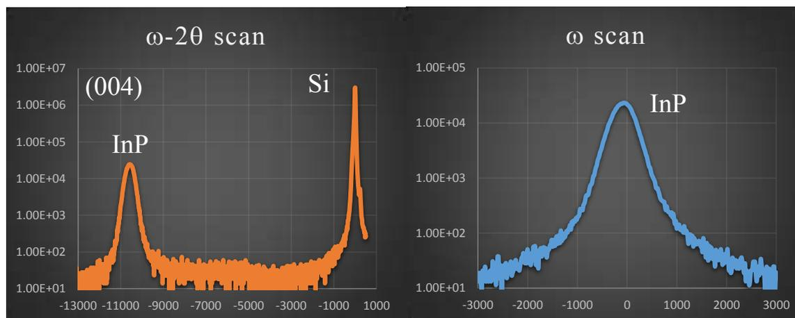
Figure 4. (a) X-ray diffraction  $\omega$ - $2\theta$  scans along the Si (0 0 4) Bragg reflection and (b) X-ray rocking curve ( $\omega$ -scans) along the InP (0 0 4) Bragg reflection of InP/Si heterostructure in patterned Si wafer.
