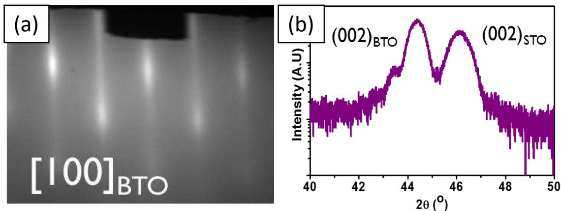
Figure 9. (a) RHEED pattern along  $[100]$  BaTiO<sub>3</sub> azimuthal direction. (b) Out-of-plane XRD  $2\theta/\omega$  measurement recorded around the BTO/STO (002) Bragg reflections
