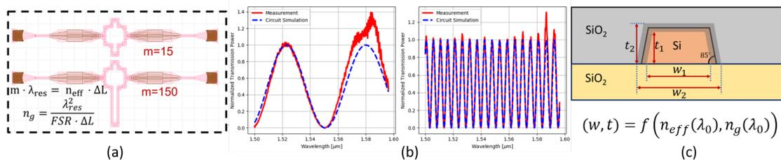
Fig. 1. (a) Two configurations of MZIs for parameter extraction. (b) Extract  $n_{eff}$  and  $n_g$  using the curve fitting method. (c) Map  $n_{eff}$  and  $n_g$  to width  $w$  and thickness  $t$ .
