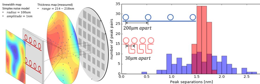
Fig. 3. (a) Generate maps of width and thickness deviation and placing ring demultiplexers over the selected points over the virtual wafer. (c) Channel spacing distribution of the demultiplexer with rings spaced 200μm apart (blue) and 30μm apart (red).
