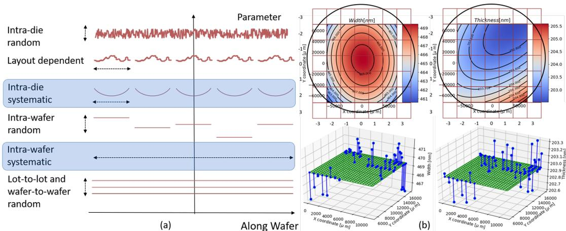
Fig. 2. (a) Illustration of decomposing spatial variability of device parameter at different levels. [6] (b) Top wafer maps of linewidth and thickness present the systematic intra-wafer variations under the process variation. Bottom wafer maps represent the systematic intra-die variations of linewidth and thickness.
