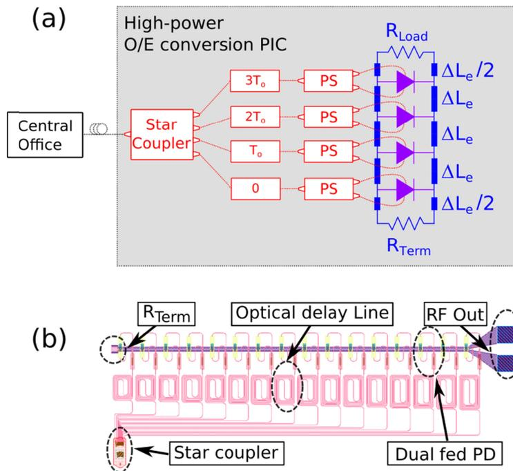
Fig. 2. Germanium traveling wave photodetector structure: (a) schematic; (b) layout of the fabricated device (PS: Power Splitter,  $T_o$ : Optical Delay,  $\Delta L_e$ : transmission line segment length).
