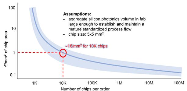
**Fig. 3.** Chip cost per mm<sup>2</sup> for silicon photonics chips in a CMOS fab, shared with nonphotonics use. The cost curve assumes that the silicon photonics volume in the fab is large enough to establish and maintain a mature process flow offering passive and active building blocks. Data are collected from the members of ePIXfab—The European Silicon Photonics Alliance (<http://epixfab.eu>).
