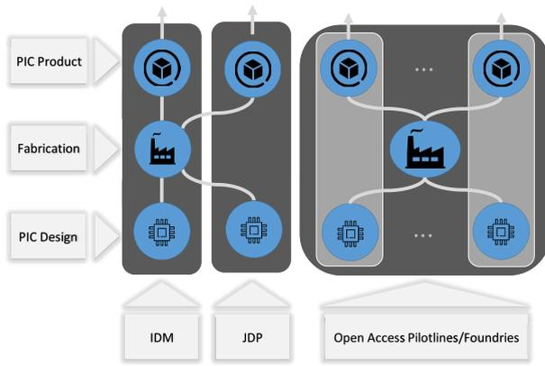
**Fig. 7.** Schematic of three prominent access models for PIC manufacturing. The first column represents vertically integrated IDMs. They internally control the entire process from chip design to production. Fabless companies can have joint development programs with IDMs as represented in the second column. The third column shows different end users submitting their PIC designs to open-access silicon photonics pilot lines/foundries for their product development.
