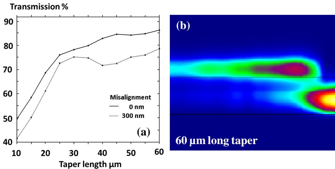
Fig. 2. (a) Simulations show the coupling from the III-V to the silicon from 10 to 60  $\mu\text{m}$  long tapers with perfect alignment of the III-V waveguide on top of the silicon waveguide, and with 300 nm misalignment, (b) the coupling from the III-V to the silicon waveguides with 60  $\mu\text{m}$  long taper and perfect alignment
