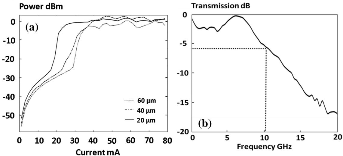
Fig. 4. (a) Power vs. current curve for fabricated lasers with 60, 40 and 20  $\mu\text{m}$  taper lengths, (b) small signal modulation showing 10 GHz 3-dB modulation bandwidth.
