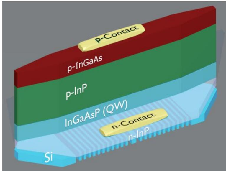
Fig. 1. 3D view of the fabricated laser showing the tapering of both the silicon and the III-V mesa
