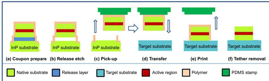
**Fig. 2** Schematic of the microtransfer print process indicating the preparation, pickup, and transfer of a single coupon from a source substrate (InP) to a target substrate.
