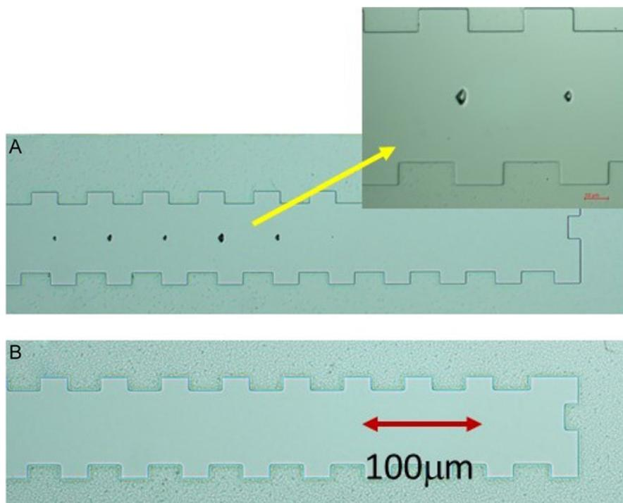
**Fig. 9** Optical images of stress induced pillars created after etching with a stressed layer on the coupon (A) and its resolution with a stress managed layer (B).
