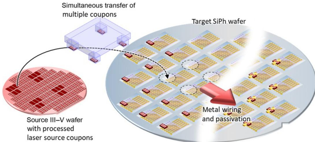
**Fig. 1** Heterogeneous integration concept for the transfer of III-V components (materials or devices such as lasers) from a source wafer to a target silicon photonics (SiPh) wafer.
