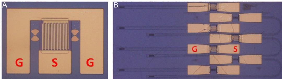
**Fig. 14** Panel (A) surface-illuminated  $70\ \mu\text{m} \times 70\ \mu\text{m}$  MSM photodetector; (B) bottom-illuminated waveguide-coupled MSM detectors. Reproduced with permission from Chen, G., Goyvaerts, J., Kumari S., Van Kerrebrouck, J., Muneeb, M., Uvin, S., Yu, Y., Roelkens G., 2018. Integration of high-speed GaAs metal–semiconductor–metal photodetectors by means of transfer printing for 850 nm wavelength photonic interposers, *Opt. Express* 26, 6351–6359. Copyright 2018 OSA.
