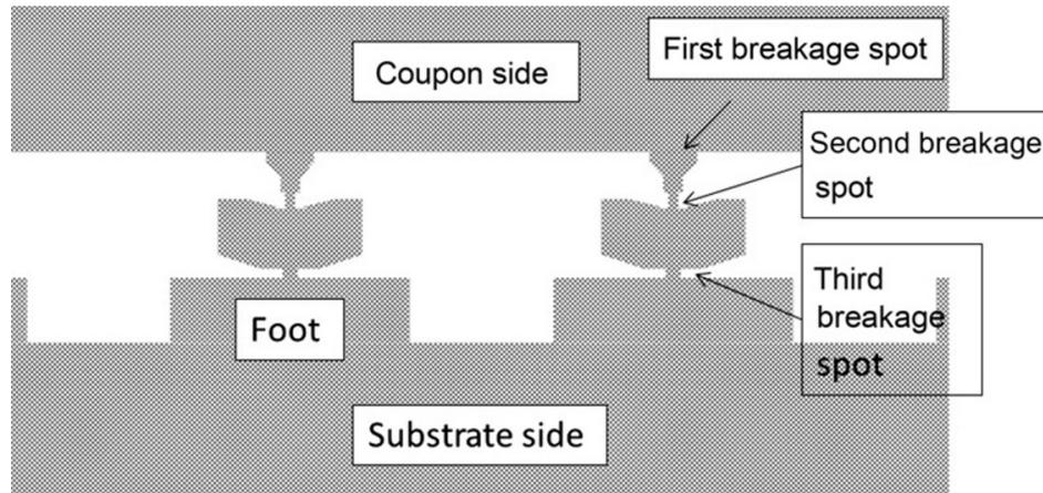
**Fig. 5** Layout example of a tether retaining a coupon in place during and after undercut etching.
