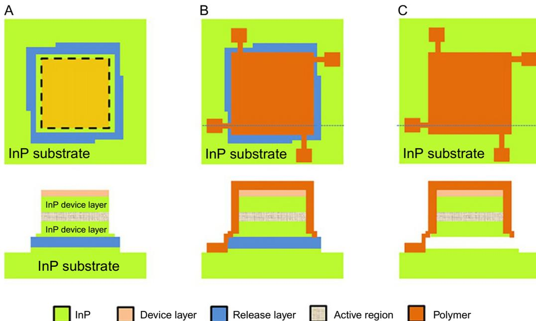
**Fig. 4** Example process preparation of InP coupons for transfer (plan and cross-section at shown location). (A) Define respective mesas for the device and the release layer. (B) Resist tethering arrangement anchors the coupons to the substrate and prevents complete sealing of the release layer. (C) The release layer is etched resulting in suspended coupons.
