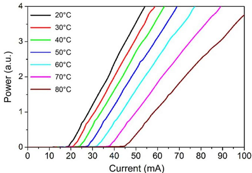
**Fig. 11** Temperature-dependent light–current characteristics of 1550 nm etched facet laser transferred to Si.
