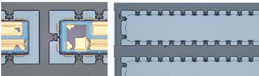
**Fig. 6** Microscope image of resist tethering system showing devices held in place after release etch and before pickup (*left*) and after device pickup showing remaining InP stub and resist anchors (*right*).
