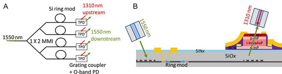
**Fig. 15** (A) Schematic layout of the III–V-on-silicon FTTH transceiver array and (B) schematic cross-section of one transceiver. TPD: transparent photodetector. Reproduced with permission from Zhang, J., et al., 2017. Silicon photonics fiber-to-the-home transceiver array based on transfer-printing based integration of III–V photodetectors. *Opt. Express* 25, 14290. Copyright 2018 OSA.
