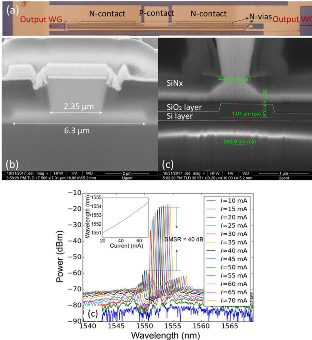
**Fig. 13** (A) Top-view of the evanescently coupled III–V-on-silicon DFB laser; (B) cross-section of the laser mesa (B) and taper tip (C); (D) output spectrum of the laser as a function of bias current. *Reproduced with permission from Zhang, J., et al., 2018. Transfer-printing-based integration of a III–V-on-silicon distributed feedback laser. Opt. Express 28, 8821–8830.*
