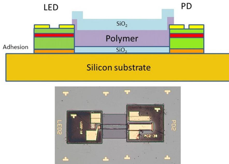
**Fig. 16** *Upper* is a schematic cross-section of the optical link containing transfer printed LED and PD while *lower* is the realized connection.
