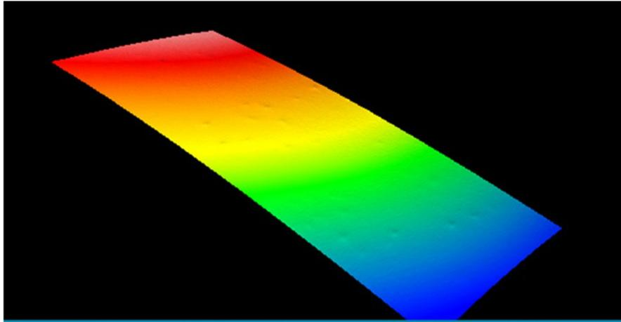
**Fig. 8** White light interferogram of the bottom side of an InP coupon after release etching of an InAlAs/InGaAs bilayer.
