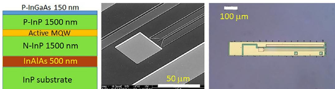
**Fig. 10** Schematic layer structure for a 1550 nm emitting laser (*left*), scanning electron microscope image of an etched facet (*center*), and optical microscope image of transferred laser prior to tether removal (*right*).
