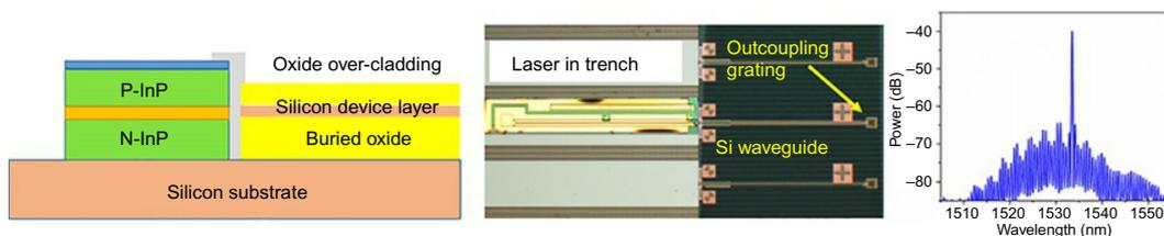
**Fig. 12** Edge geometry for laser–waveguide coupling (*left*) using microtransfer printing, optical image of laser printed with respect to the waveguide (*center*), and outcoupled spectrum from grating (*right*).
