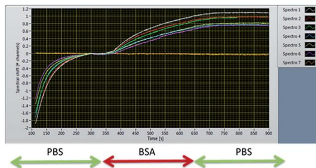
Fig. 13 Physical adsorption of BSA using an unfunctionalised cartridge.
