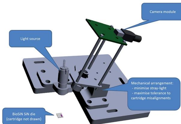
Fig. 11 Optical readout module (upside down).
