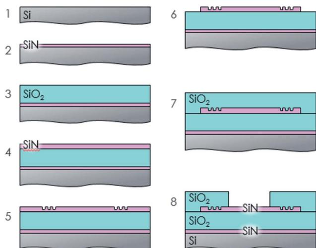
Fig. 4 Process flow for the SiN photonic chip fabrication. (1) Si substrate, (2) deposition of the anti-reflective coating, (3) deposition and chemical-mechanical polishing (CMP) of the bottom clad, (4) deposition of the SiN waveguide layer, (5) shallow etch of the grating couplers, (6) deep etch of the waveguides, (7) deposition and CMP of the top clad, and (8) clad-open etch.
