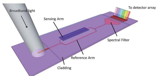
Fig. 1 Integrated photonic sensor circuit consisting of a MZI sensor read-out by an on-chip AWG spectral filter.
