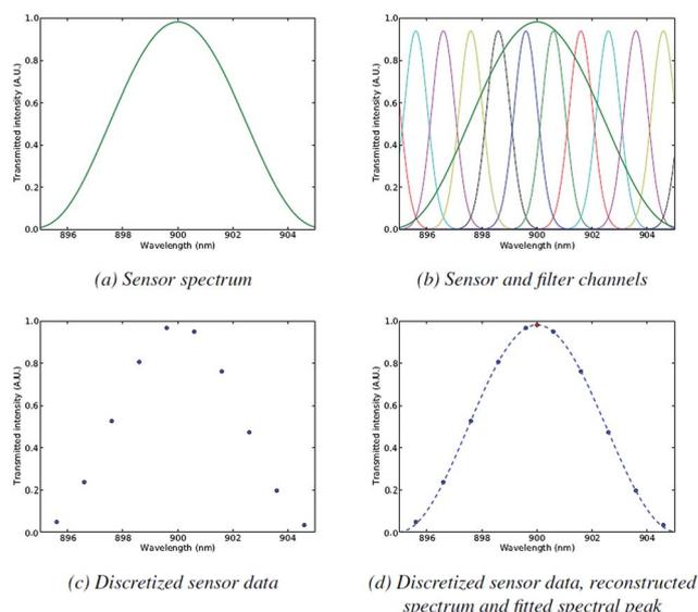
Fig. 2 Interrogation principle based on a broadband source and an on-chip spectral filter.
