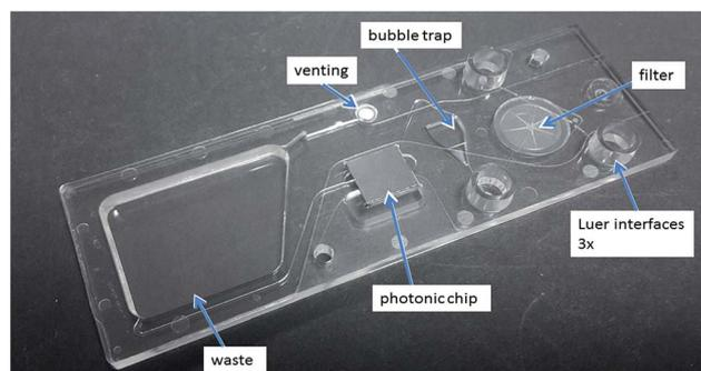
Fig. 8 Assembled microfluidic cartridge.
