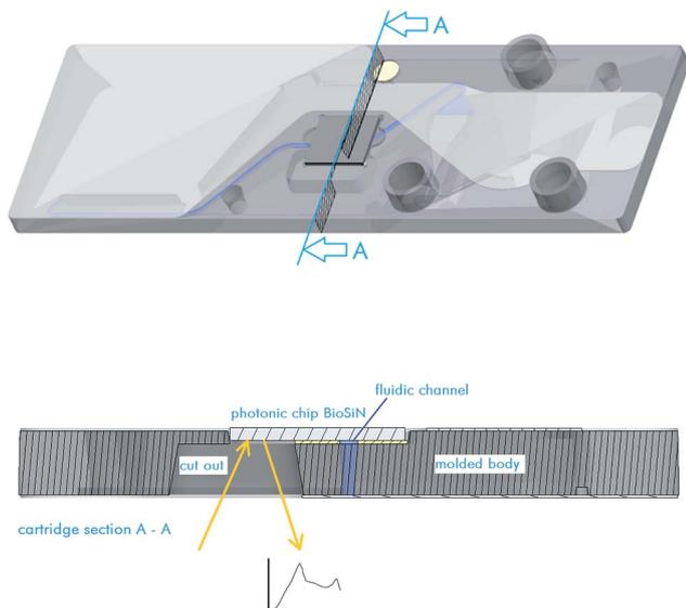
Fig. 9 Cross section (bottom) through the microfluidic cartridge along section A–A (indicated in the top figure).
