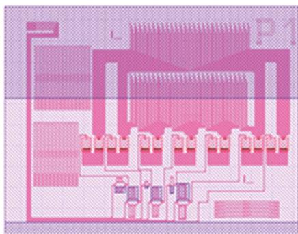
Fig. 3 Layout of a sensing circuit consisting of 6 sensors, each of them with their own MZI and AWG.
