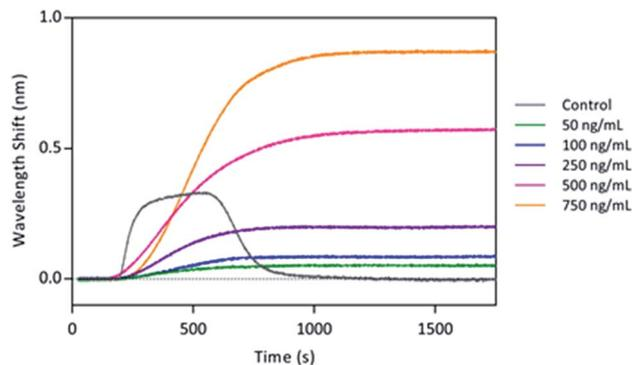
Fig. 14 Real-time monitoring of different CRP concentrations and BSA as a control with the biosensor instrument.
