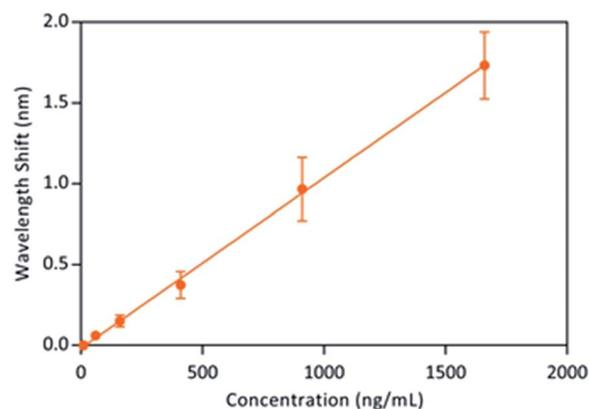
Fig. 15 Calibration curve for the detection of CRP in PBS.
