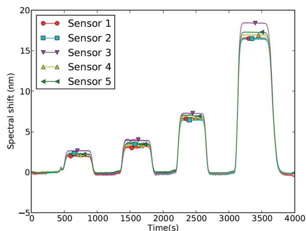
Fig. 5 Sensorgram of parallel measurement of five MZI sensors, where the sensors are exposed to different concentrations of HCl in alternation with water.
