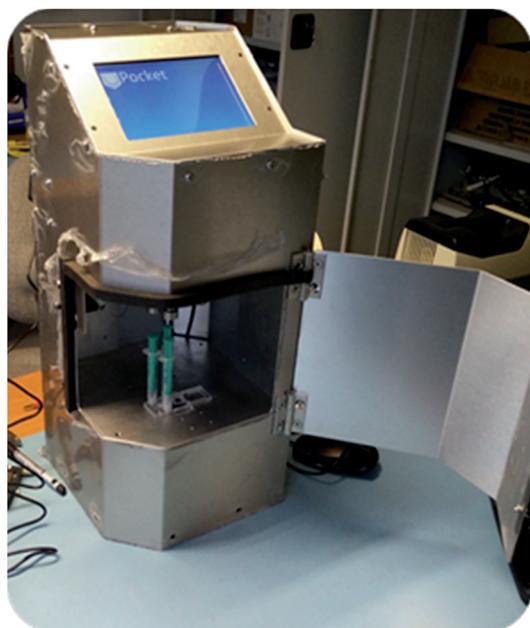
Fig. 10 Integrated readout instrument.
