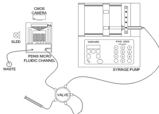
Fig. 6 Experimental setup of the lab-based prototype.
