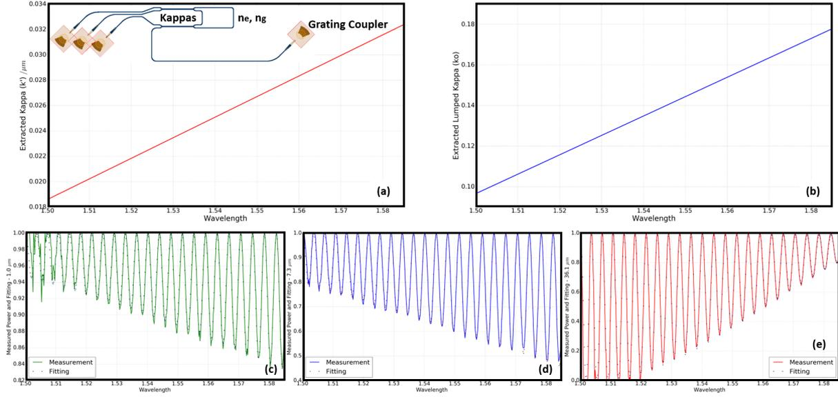
Figure 3. (a) Extracted field coupling coefficients ( $\kappa'$ ) from the MZI. (b) Extracted lumped coupling coefficient ( $\kappa_0$ ). (c,d,e) Measured and the fitted spectra from the coupled spectra of the MZI structures with coupling lengths 7.3, 36.1 and 1.0  $\mu\text{m}$  respectively.
