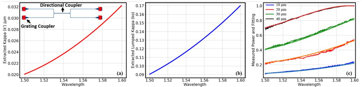
Figure 2. (a) Extracted field coupling coefficient using a 'naked' directional coupler. (b) Extracted lumped coupling coefficient. (c) Measured and the fitted spectra from the coupled port of the directional couplers with coupling lengths of 10, 20, 30 and 40  $\mu m$ .
