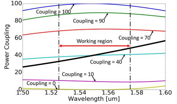
Fig. 4. The simulated cross power transmission for 0%, 10%, 40%, 70%, 90% and 100% coupling ratio. Within the working region between  $1525 \text{ nm}$  and  $1575 \text{ nm}$  indicated by the dashed line, the device works as a broadband coupler with a deviation less than 3%. Outside this working region, the coupler suffers more wavelength dispersion. The dispersive response of a single DC with 40:60 coupling ratio at  $1550 \text{ nm}$  is also shown by black bold line.
