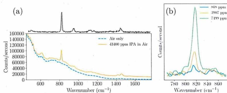
Fig. 2. (a) The Raman spectra before (blue dashed line) and after (orange solid line) the application of saturated IPA vapor. Reference Raman spectra from pure liquid IPA is also given (black dotted). (b) The background-subtracted Raman spectra of the  $819\text{ cm}^{-1}$  mode at various concentrations.
