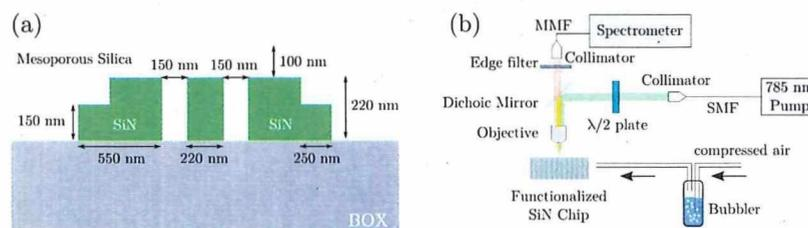
Fig. 1. (a) The cross-section of the double-slot SiN waveguide. (b) The setup for VOC experiments. The backward-propagating Raman signal is measured and the VOC vapor is prepared by a bubbler.
