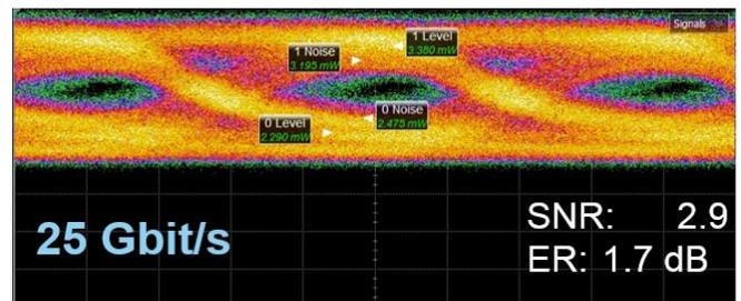
Fig. 2 Optical  $2^7-1$  PRBS eye diagrams measured at 1560 nm, with a drive voltage of  $2.5 V_{pp}$  and a voltage bias of 2 V, at 25Gbit/s.
