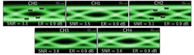
Fig. 5 Eye diagrams measured at 25 Gbit/s on the 5 channels of a WDM transmitter with  $W_{wg} = 600$  nm and  $L_{device} = 100 \mu$ m at 2.5  $V_{pp}$  and -1.2 V DC bias.
