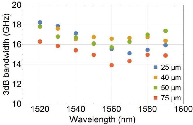
Fig. 3 3dB bandwidth measured at 0 V DC bias from 1520 nm to 1600 nm on graphene EAMs with lengths of 25 $\mu$ m, 40 $\mu$ m, 50 $\mu$ m and 75 $\mu$ m.
