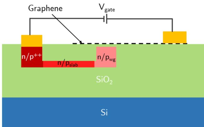
Fig. 1 Schematic cross section of the graphene EAM.
