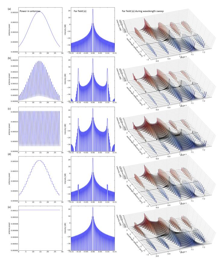
Fig. 7. Different power distribution profiles for the pixelated dispersive OPA, the resulting far field profile when all the antennas are in phase, and the evolution of the far-field when sweeping the wavelength. (a) Gaussian profile over all antennas, as used in Fig. 6. (b)–(e) Different combinations of Gaussian and Uniform distributions within a block and between blocks. All power distributions are normalized for unity power.
