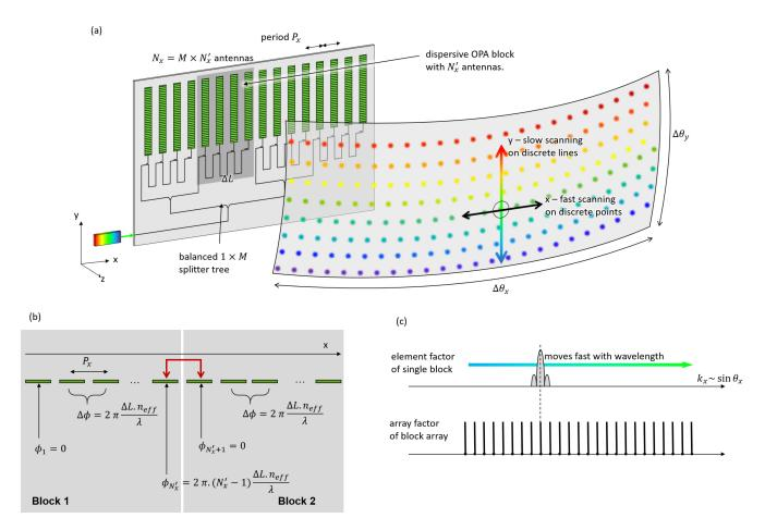
Fig. 5. Discretized dispersive optical phased array. (a) Schematic structure, where each block consists of a snake-like OPA. It is also possible to use a Tree or AWG-like OPA in each block. (b) Condition when all antennas are in phase, and (c) overlap of scanning beam of single block with diffraction orders of the large array.
