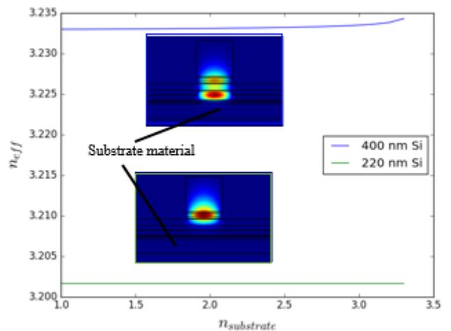
Figure 2: Effective index of the etched and unetched parts of the DFB grating that forms the laser cavity as a function of the substrate index.
