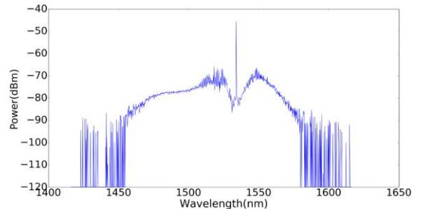
Figure 4: spectrum of the two-step transfer printed DFB laser on a LN platform with 90 mA pump current
