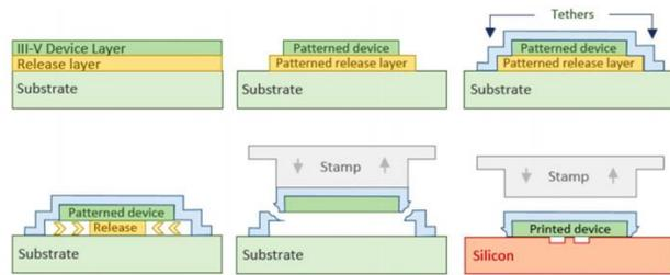
Figure 1: Cross sectional view of the transfer printing of III-V coupons on a silicon substrate
