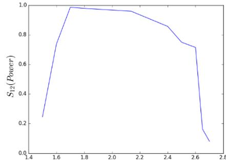
Figure 3: power coupling of the taper we designed for different substrate indexes
